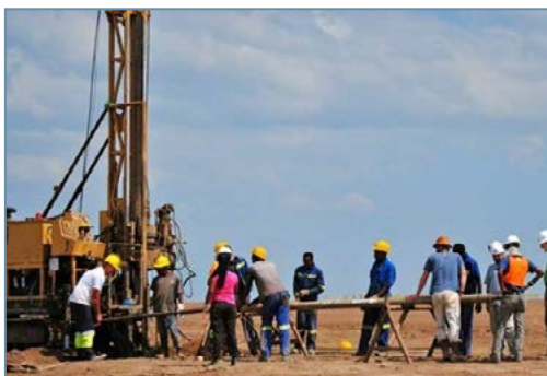
The Chew Bahir Drilling Project: Preparing to remove a core section in its core liner from the lowermost drill rod © Verena Foerster, University of Potsdam
