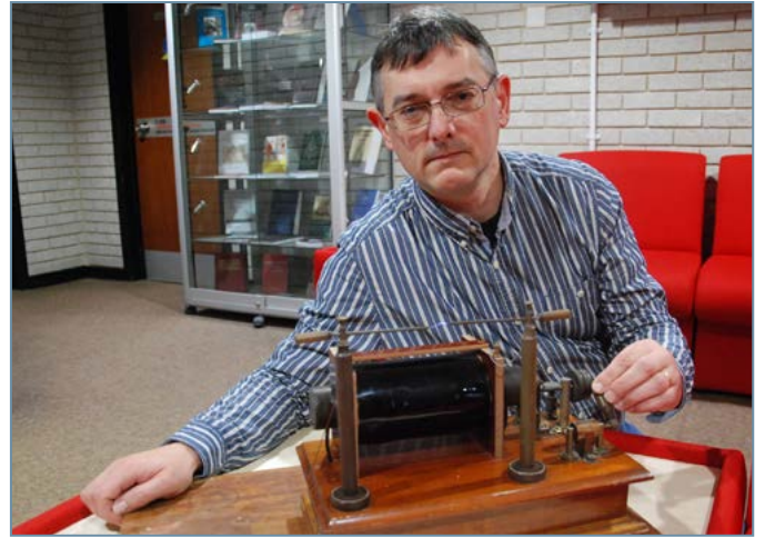
Professor Iwan Morus with an induction coil which was in use from the 1830s. Between around 1890 and 1920 these were used to generate high voltage to create electromagnetic (radio) waves.
