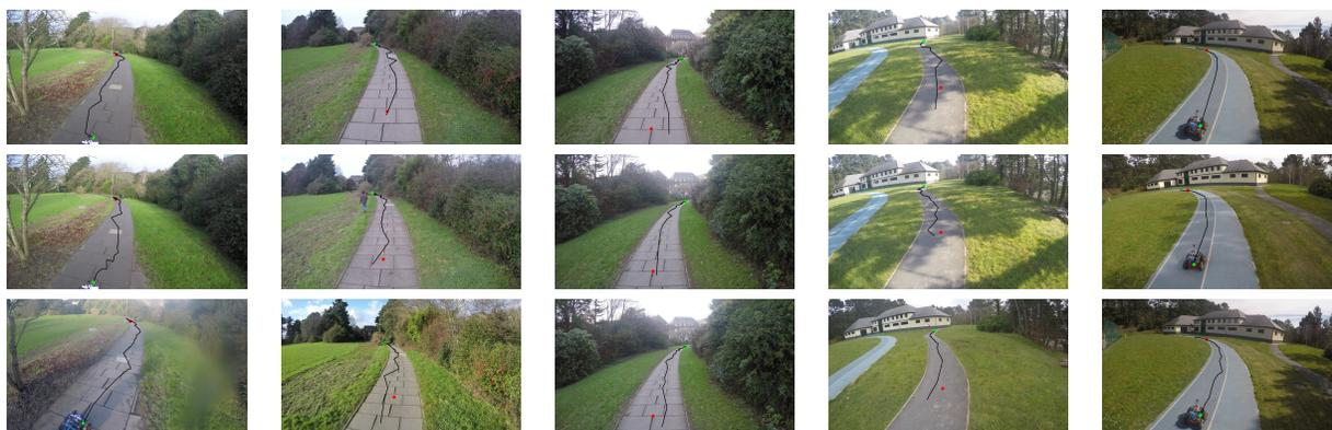
Fig. 7. Outdoor environments. The black line refers to the robot's trajectory, green dot the starting position and red dot the end position of the trial. Images in the topmost, middle and bottom rows correspond to trials carried out with the ASH, USH and BUV colour models (respectively).
