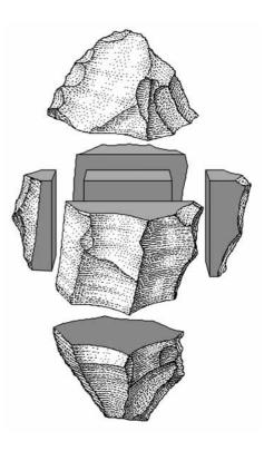
Fig 30 Removing the outer surfaces of a burnt flint with a diamond saw – the inner core is crushed and the material used to measure luminescence (diagram courtesy of Dr N Debenham).
