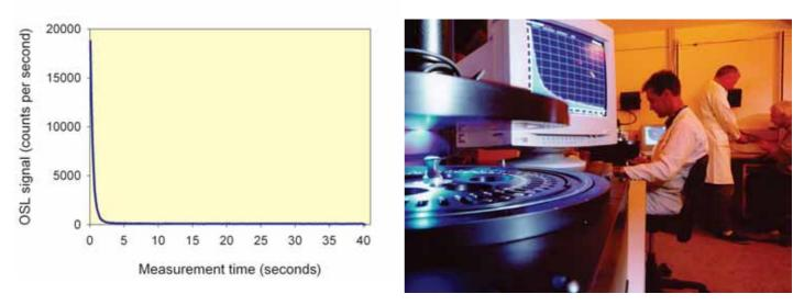
Fig 6 (left) Typical OSL signal observed from a quartz aliquot – the OSL signal drops rapidly as the trapped electrons in the quartz are used up to produce the luminescence signal. (right) An automated luminescence reader equipped with blue-light-emitting diodes (LEDs). When in use, the lid closes, leaving the sample holder in darkness. The blue LEDs are switched on to measure the optically stimulated luminescence (OSL) signal (© Risø National Laboratory, Denmark).
