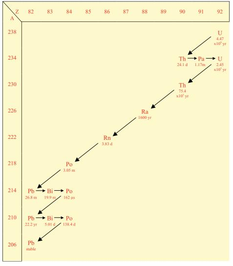
Fig 23 The decay chain of <sup>238</sup>U: arrows show the sequence of isotopes produced by emission of a beta particle (horizontal arrows) or an alpha particle (diagonal), with half-lives varying from hundreds of thousands of years to less than a second (Z = atomic number, the number of protons in the nucleus and hence chemical properties; A = atomic mass (sum of protons and neutrons), which differentiates isotopes).
