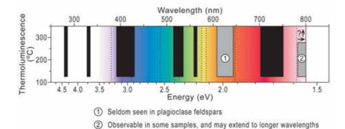
Fig 10 Quartz (above) and feldspars (below) emit luminescence at wavelengths ranging from ultraviolet through visible into infrared – dark bands show the strongest emissions. Quartz shows clear TL peaks – some are stable through geological time and found in natural samples; others are relatively short-lived (peaks >  $200^{\circ}$ C) and only found in artificially irradiated samples (modified from Stokes and Fattahi 2003).
