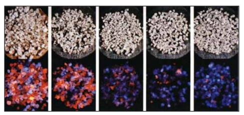
**Fig 9** (upper row) Five quartz samples shown in room-light conditions (each metal disc = 9.8mm diam; quartz grains c 0.2mm diam). (lower row) Image, taken using highly sensitive photographic paper; of the thermoluminescence (TL) signal emitted by the grains being heated. Some grains emit most strongly in the orange–red part of the spectrum; others are strongest in the blue (from Hashimoto *et al* 1986).
