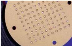
Fig 20 (top) Luminescence measurements made by focussing a green laser beam on the sample (beam diam *c* 0.02mm when it strikes a grain). (bottom) Individual quartz grains (0.2mm diam) held in an array of 10 × 10 holes drilled in the surface of the 9.8mm diam sample holder. The laser beam is moved using mirrors to strike one grain at a time, giving an OSL signal (@ Risø National Laboratory, Denmark).
