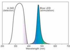
**Fig 11** Blue LEDs, with emission centred at *c* 470nm, create a very bright source of light used to stimulate an OSL signal from quartz. The luminescence signal emitted from a sample is typically a million million (ie 1,000,000,000,000) times weaker than the LEDs. Such a weak signal is detected using a photomultiplier tube (PMT), filtering the PMT from the blue LEDs with a Hoya U-340 (which blocks light wavelengths > *c* 380nm).
