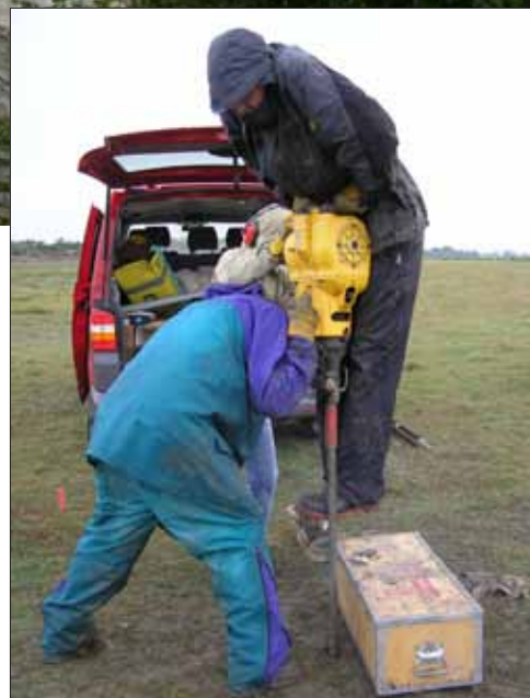
Percussion-coring in inclement weather, near Faeceni, SE Romania.
