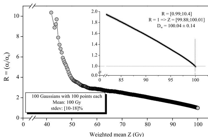
Figure 7.6: The ratio  $R$  between the internal estimate of uncertainty  $\alpha_{in}$  and the external estimate of uncertainty  $\alpha_{ex}$  is plotted against the weighted mean for a simulated Gaussian distribution.
