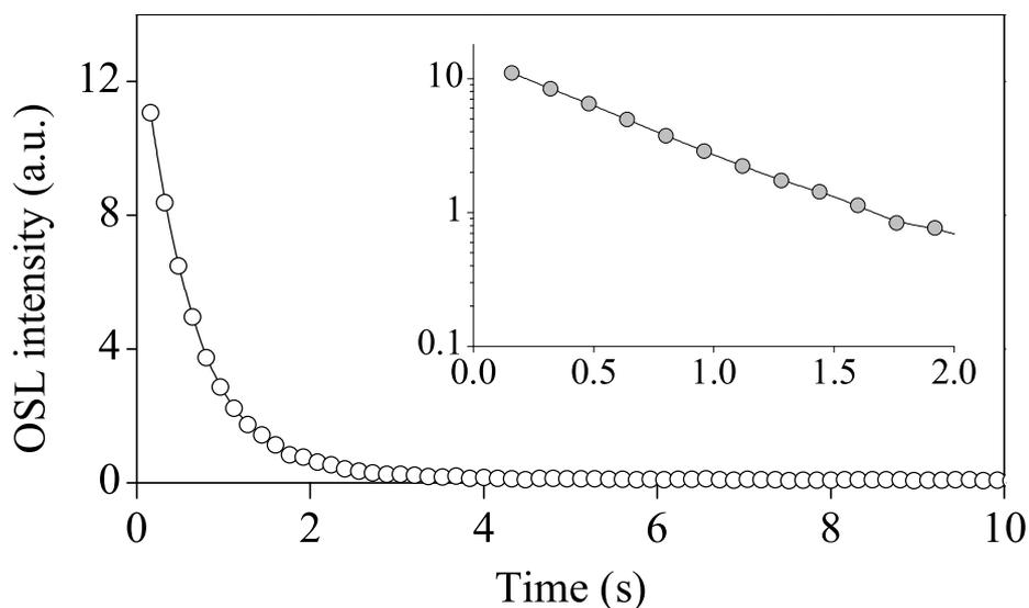
Figure 3.4: A CW-OSL decay curve obtained from a sedimentary aeolian quartz sample (lab code: 010414). The sample was stimulated using blue LEDs and the luminescence detected through 7.5 mm Hoya U-340 filters. Inset: same data as the graph but shown on a log scale. The initial part of the decay in this sample can be fitted adequately by a simple decaying exponential function. Note the logarithmic scale.
