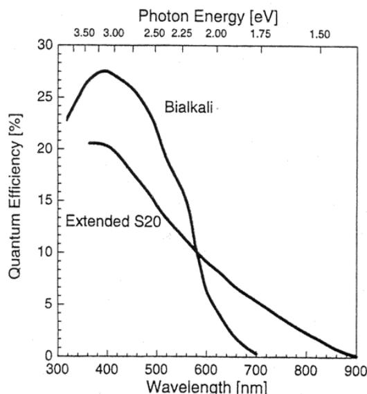
Figure 4.2: The quantum efficiency of the photomultiplier tubes EMI 9235QA PMT (Bialkali) and EMI 9658R PMT (Extended S20) as a function of photon wavelength and energy; (from Bøtter-Jensen, 1997).
