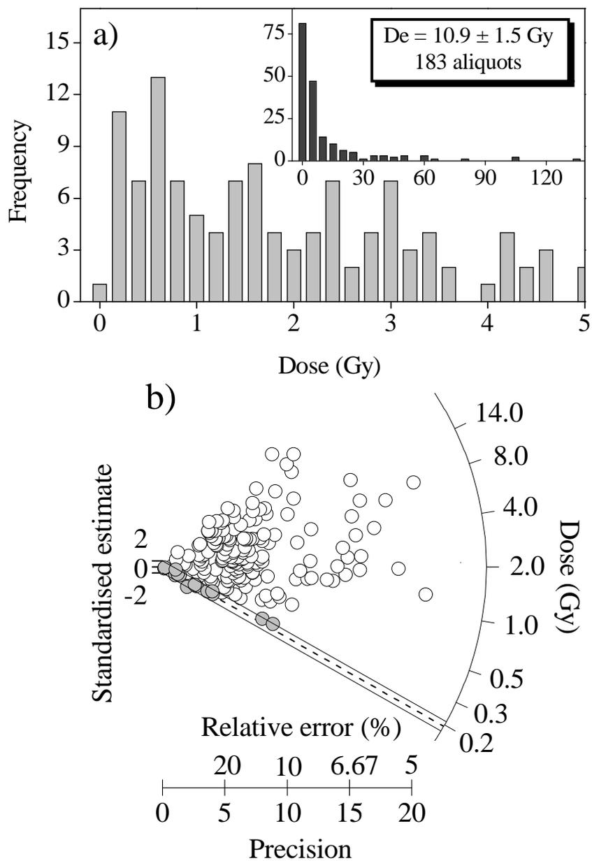
Figure 5.3: Doses measured in small aliquots of quartz extracted from unirradiated concrete. **a)** Histogram, using only those results with a natural test dose known to better than 15% ( $n = 183$ ); the arithmetic average is given in the inset. **b)** Radial plot, showing the results selected for inclusion in the average result of  $0.28 \pm 0.05$  Gy ( $n = 18$ ).
