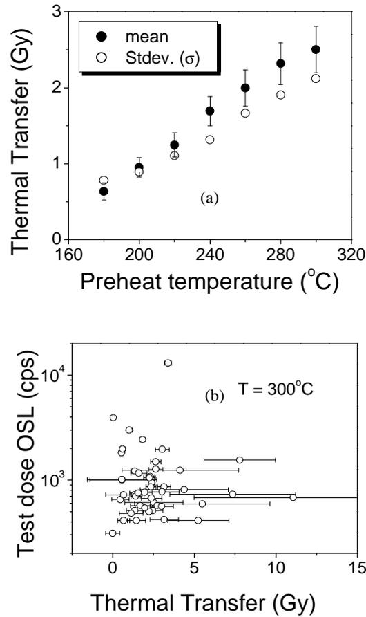
Figure 8.2: **a)** A plot of mean and standard deviation of the thermal transfer for each preheat temperature. The error bars on the mean values are the standard errors. **b)** A scatter plot of the cumulative thermal transfer at  $300^{\circ}\text{C}$  versus the first test dose OSL response of the each grain.
