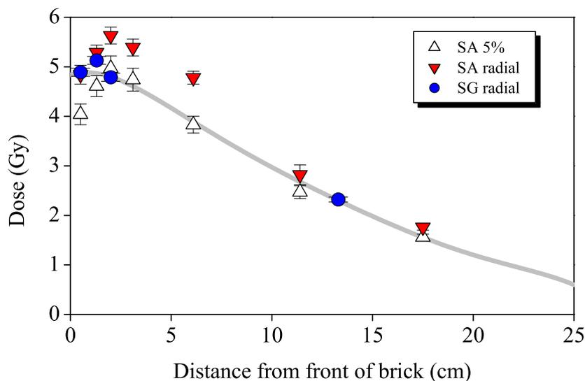
Figure 5.8: Comparison of small aliquot (SA) results derived from the first 5% of histograms (triangles), radial plots (inverted triangles) and single grain (SG) results (circles) with the predicted depth-dose curve.
