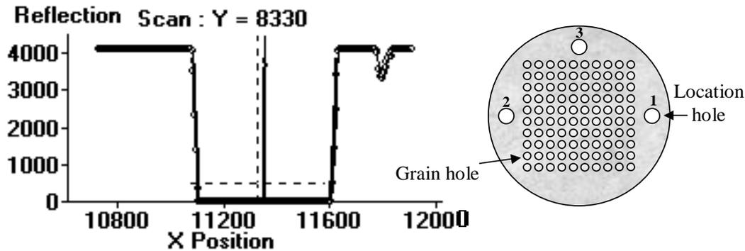
Figure 4.13: Example of a location hole scan. The change in reflectivity as the laser passes over the location hole is clearly seen. The diameter of the location hole is  $500\ \mu\text{m}$  as expected. Also shown is a schematic drawing of a single grain disc.
