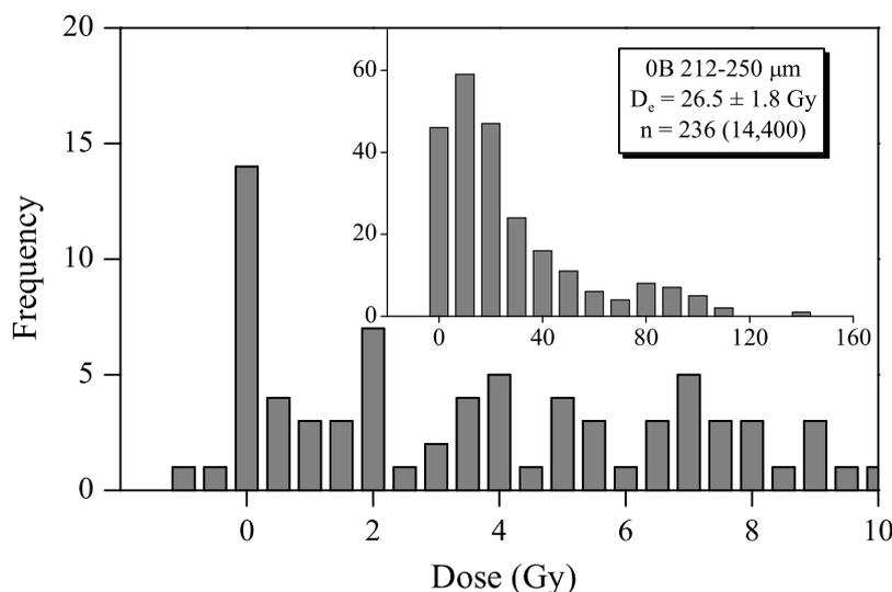
Figure 7.1: Natural doses measured from single grains of quartz (212 – 250  $\mu\text{m}$  fraction) extracted from an unirradiated portion of the bulk concrete. All results included in the figure have uncertainties on the natural test dose, based on photon counting statistics, of  $< 20\%$ . The average dose is  $26.5 \pm 1.8$  Gy ( $n = 236$ ).
