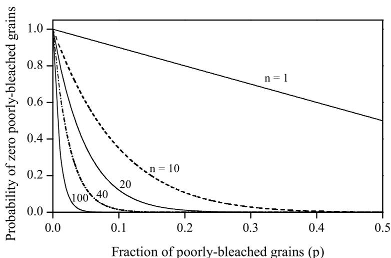
Figure 3.10: Probability of including only well-bleached grains in an aliquot consisting of  $n$  grains as a function of the fraction of poorly-bleached grains in the sample. Based on Figure 4 in Olley et al. (1999).
