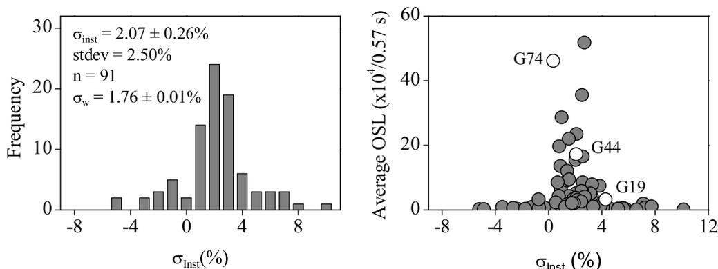
Figure 4.21: Assessment of the single grain attachment instrument reproducibility using test-dose corrected OSL signals and the first 0.57 s of stimulation. a) Frequency histogram of the individual estimates of instrument reproducibility  $\sigma_{inst}$ . b) The average integrated OSL signal as a function of the individual estimates of the instrument reproducibility.
