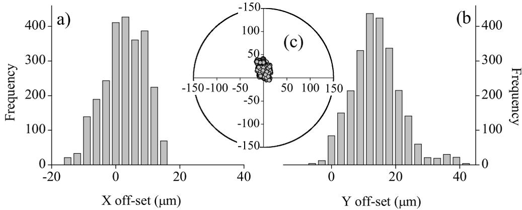
Figure 4.16: Accuracy and precision of the location routine in locating individual grain holes. The grain hole search routine was repeated 2,500 times. **a)** Frequency histogram of the off-set on the x-axis. **b)** Frequency histogram of the off-set on the y-axis. **c)** The off-sets on the y-axis as a function of the corresponding off-sets on the x-axis. The circle represents the dimensions of a grain hole.
