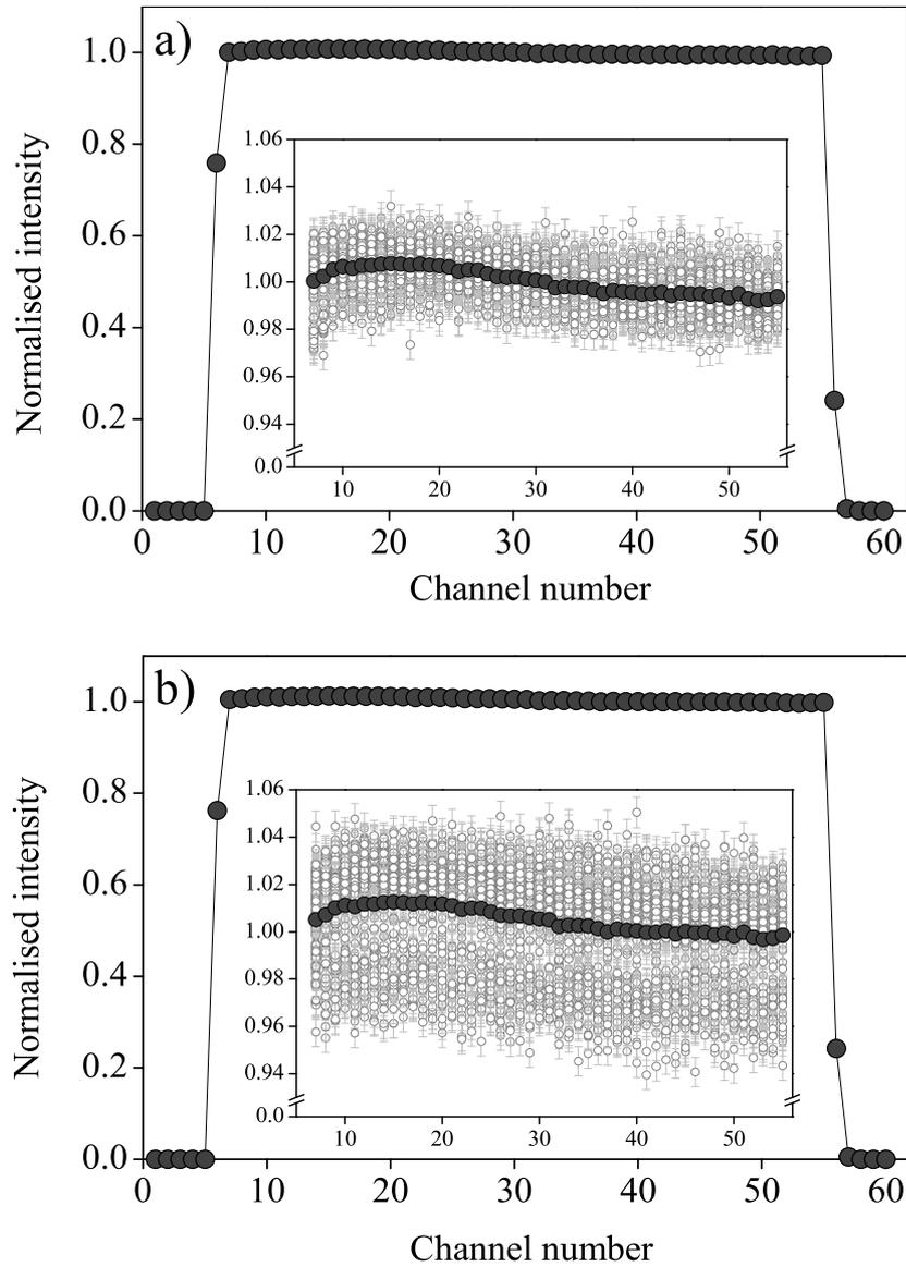
Figure 4.10: Reproducibility of the green laser. The average normalised light intensity as a function channel number. **a)** The data have been normalised to the average intensity of each stimulation (channel 7–55). **b)** The data have been normalised to the average intensity of all measurements (channel 7–55).
