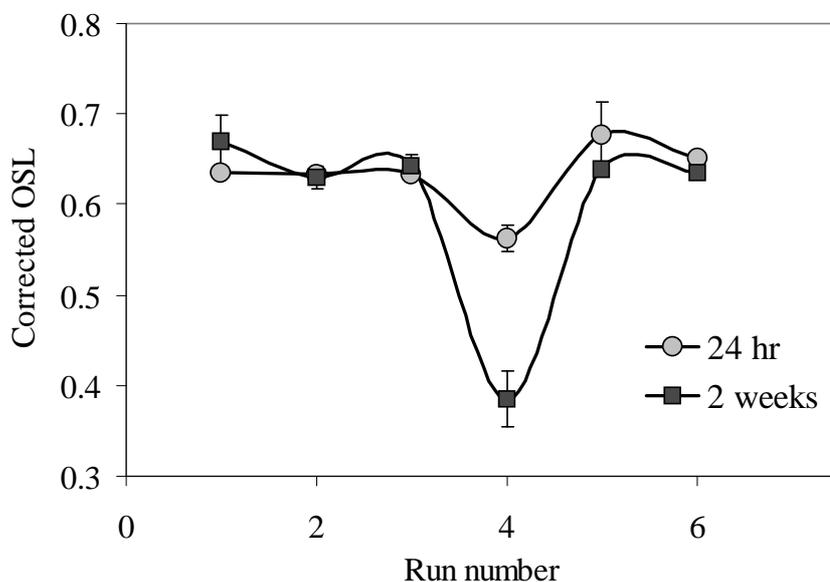
Figure 9.3: Fading data for Blue care<sup>®</sup>. Each point is an average of two aliquots. The samples were dosed and stored for either 24 hr or 2 weeks at ambient temperature. Prior to storage, three SAR measurement cycles were carried out (run 1, 2 and 3), each time giving the same dose (regeneration dose: 1 Gy, preheat temperature: 150 °C for 10 s, test dose: 0.5 Gy, no cutheat). After storage the same three measurement cycles were carried out (run 4, 5 and 6).
