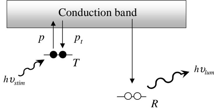
Figure 3.6: Energy level diagram of the simple General One-Trap (GOT) model. An electron captured in the trap  $T$  is optically excited into the conduction band. The released electron will either be retrapped in  $T$  or recombine in the radiative recombination centre  $R$ , whereby a photon is emitted.
