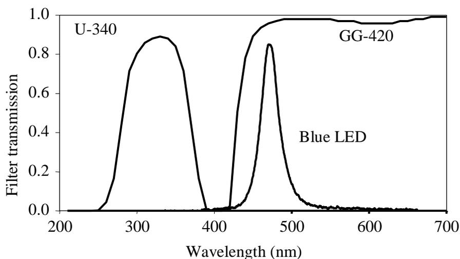
Figure 4.5: The emission spectrum of blue LEDs. Also shown are the transmission curves for the GG-420 green long pass filter (cut-off filter in front of the blue LEDs) and the Hoya U-340 filter (detection filter in front of the PMT); after Bøtter-Jensen et al. (1999b).
