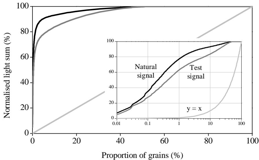
Figure 5.9: Cumulative light sum against proportion of contributing grains for natural and test dose signal obtained from the 12,000 grains measured from slice 1. The line  $y = x$  represents an “ideal” sample where all grains contribute equally to the light sum.
