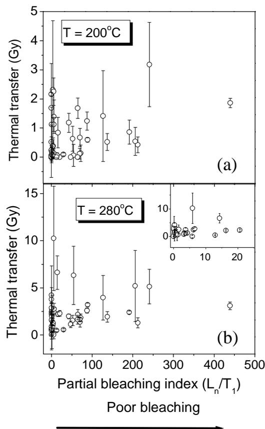
Figure 8.3: Relationship between thermal transfer and the extent of partial bleaching in individual grains for preheat temperatures of **a)** 200 °C and **b)** 280 °C.
