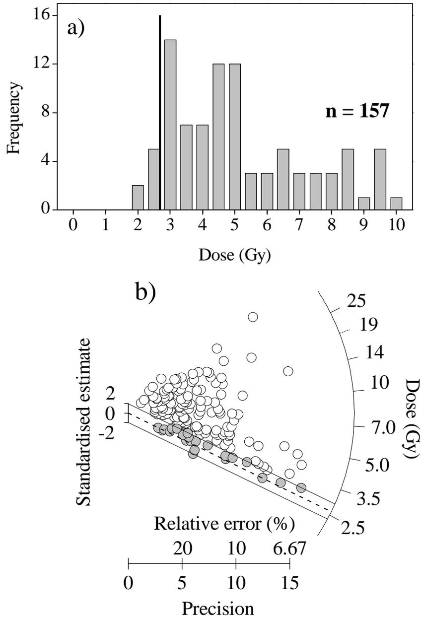
Figure 5.5: Doses measured in small aliquots of quartz extracted from slice 12 (11.4 cm into the brick) of the simulated brick (expected dose  $2.68 \pm 0.02$  Gy). **a)** Histogram, using only those results with a natural test dose known to better than 15% ( $n = 157$ ); the vertical black line represents the expected dose. **b)** Radial plot, showing the results selected for inclusion in the average result of  $2.92 \pm 0.09$  Gy ( $n = 22$ ) and a weighted mean of  $2.79 \pm 0.11$  Gy .
