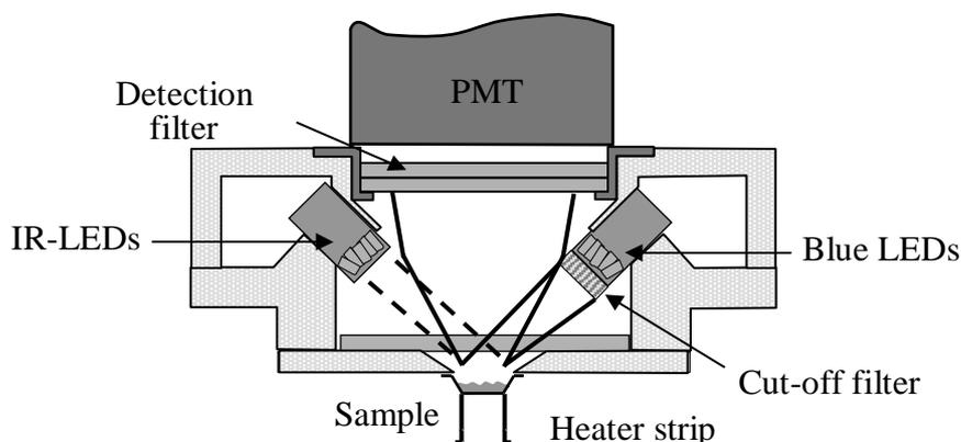
Figure 4.4: Schematic diagram of the combined blue and IR LED OSL unit. The unit contains 28 blue LEDs (in 4 clusters) emitting at 470 nm delivering  $\sim 40 \text{ mW/cm}^2$  at the sample and 21 IR LEDs (in three clusters) emitting at 875 nm delivering  $\sim 135 \text{ mW/cm}^2$  at the sample.
