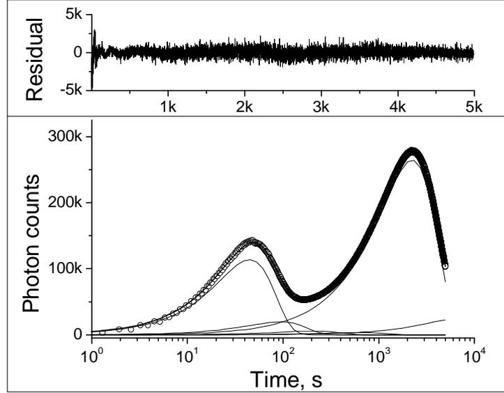
Figure 3.5: An example of a LM-OSL curve from a sensitised (heated to 700 °C) and irradiated quartz sample from Denmark. The sample was stimulated using blue LEDs and the luminescence detected through 7.5 mm Hoya U-340 filters. The LM-OSL consists of 6 exponential components. The upper graph shows the difference (residual) between the data and the fitted values. From Jain et al. (2003a).
