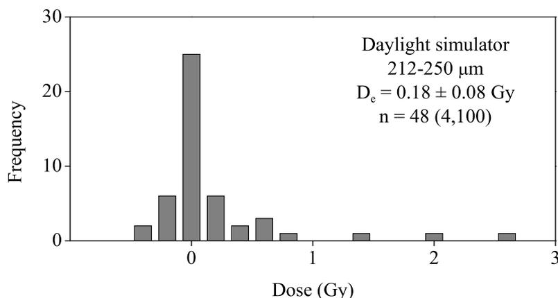
Figure 7.3: Dose histogram showing the results obtained from the portion of the bulk unirradiated sample, which was bleached under a daylight simulator for 1 hour. The average dose is  $0.18 \pm 0.08$  Gy ( $n = 48$ ).
