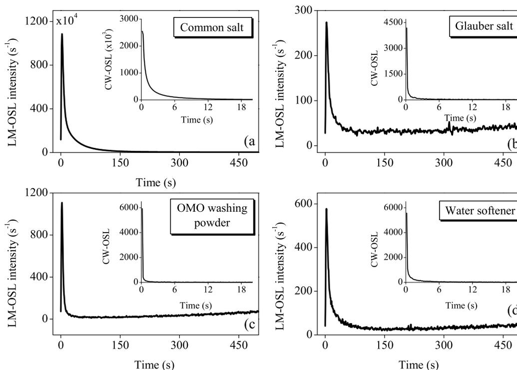
Figure 9.1: LM-OSL curves for four common household chemicals, with stimulation power increased from 0 to 100% in 500 s. The inserts show CW-OSL decay curves, measured at a constant 100% of stimulation power. The samples were given a dose of approximately 2 Gy and preheated to 150 °C before stimulation
