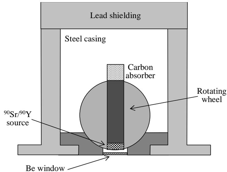
Figure 4.7: Schematic diagram of the cross section of the beta irradiator. The  $^{90}\text{Sr}/^{90}\text{Y}$  source is placed in a rotating stainless steel wheel, which is pneumatically activated. The source is shown in the *on* (irradiating) position. When the source is *off* the wheel is rotated  $180^\circ$ , so that the source points directly at the carbon absorber.
