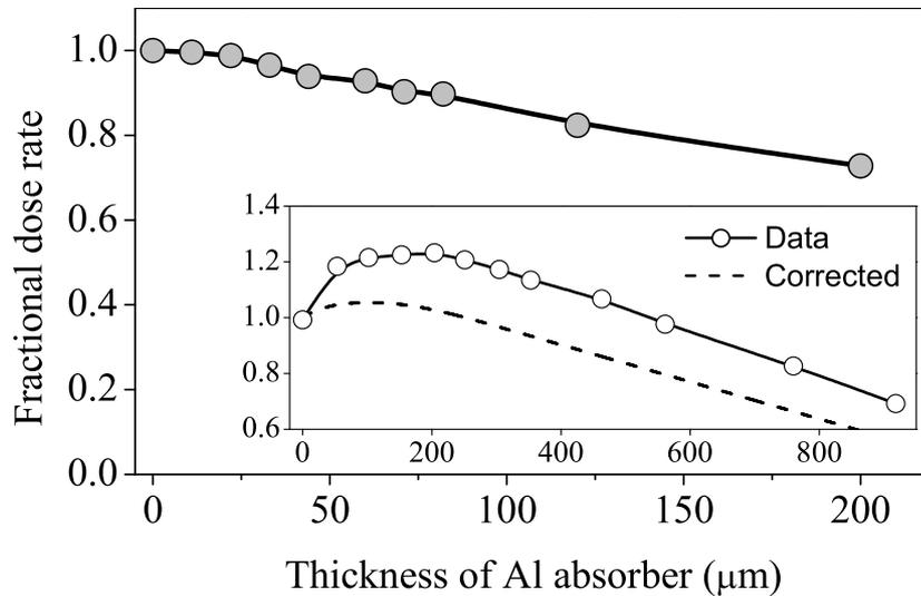
Figure 6.7: Fractional dose-depth curve measured using the Risø reader using blue LEDs and 212–250  $\mu\text{m}$  grains in single grain discs. The inset shows the data obtained by Wintle and Murray (1977) and the same data averaged over a mean path length of 133  $\mu\text{m}$ . See text for details.
