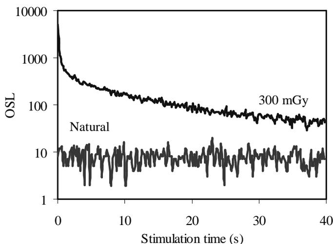
Figure 9.5: The measured natural OSL signal for Blue care<sup>®</sup> dish washing powder compared to that obtained by giving the sample a dose of 300 mGy in the laboratory.
