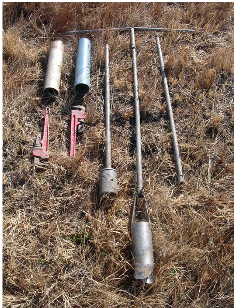
Figure 2.10: Equipment used for augering samples, showing sample tubes on the left and the various augering equipment used.
