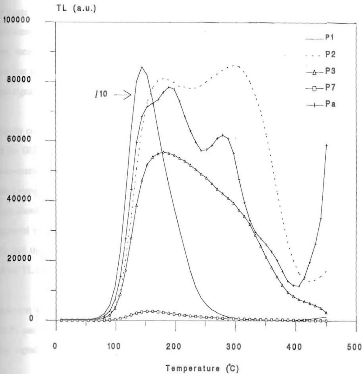
Figure 3.2.3. TL glow curves of plagioclase feldspars. TL of sample P<sub>1</sub> was reduced by a factor of 10.
