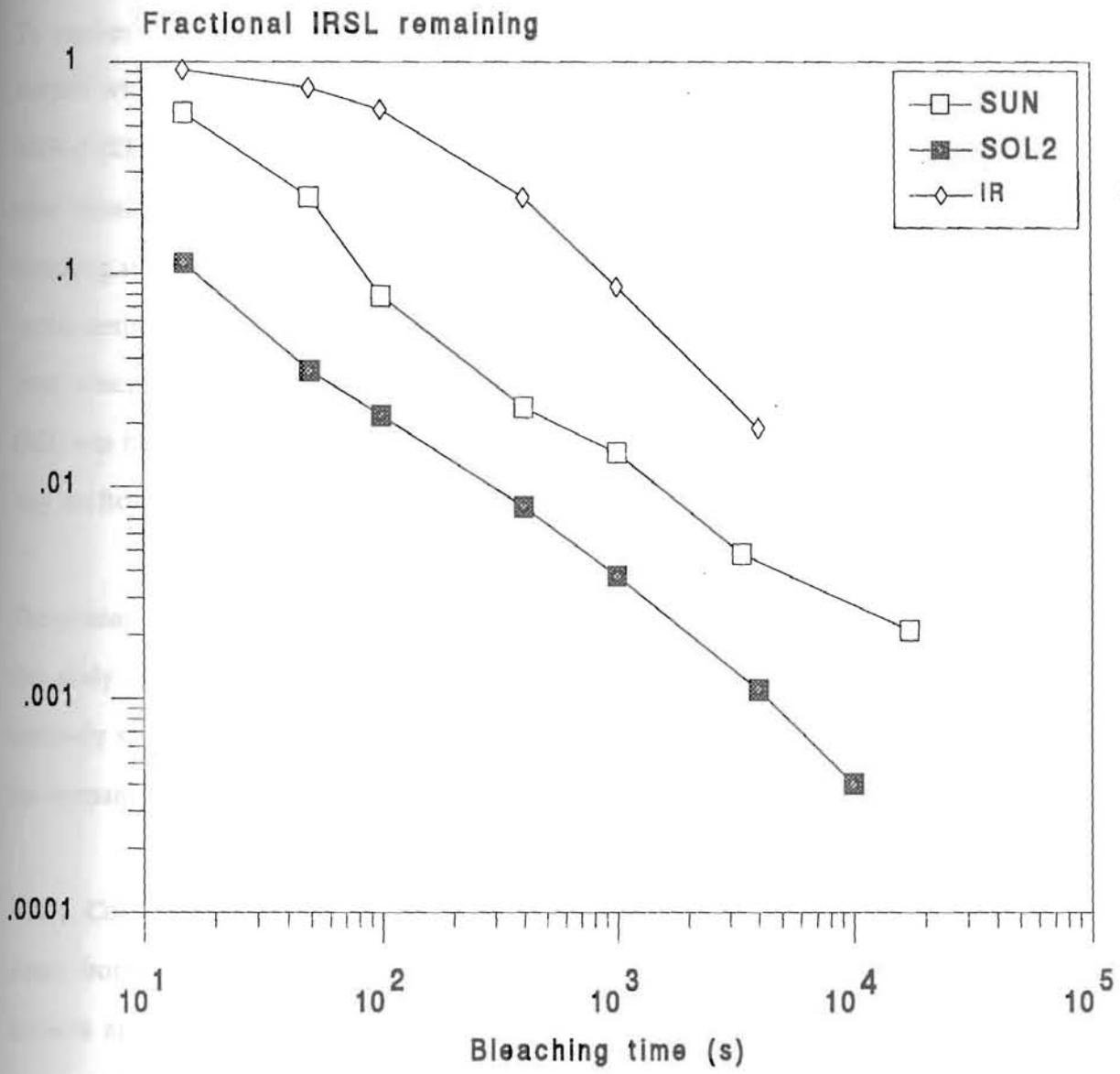
Figure 6.2.2. Comparative results of IRSL bleaching with IR, sunlight and SOL2 solar simulator.
