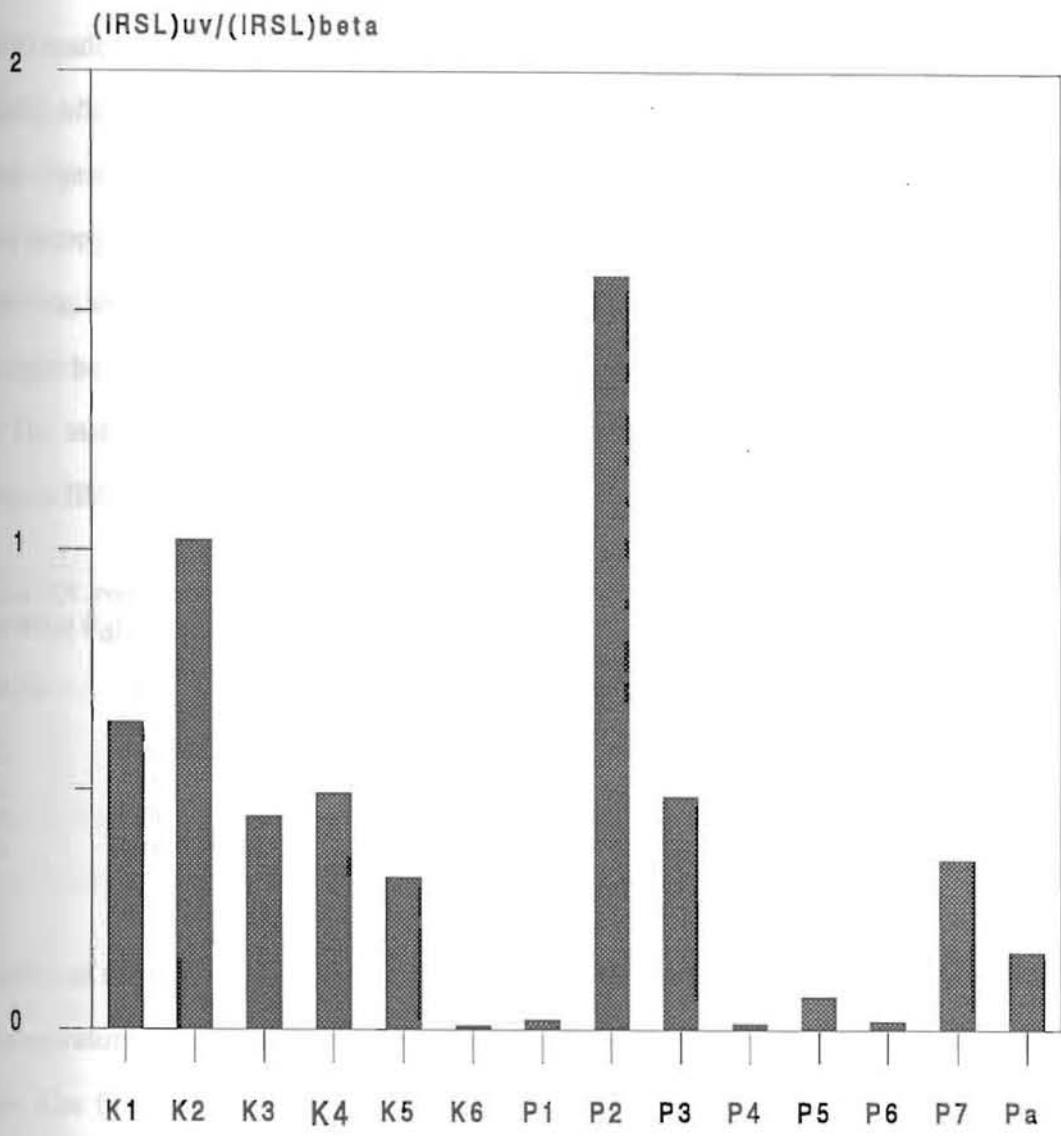
Figure 3.2.15. Ratio of u.v. (1 hour) regenerated IRSL signal and IRSL created by a  $\beta$  dose (20 Gy).
