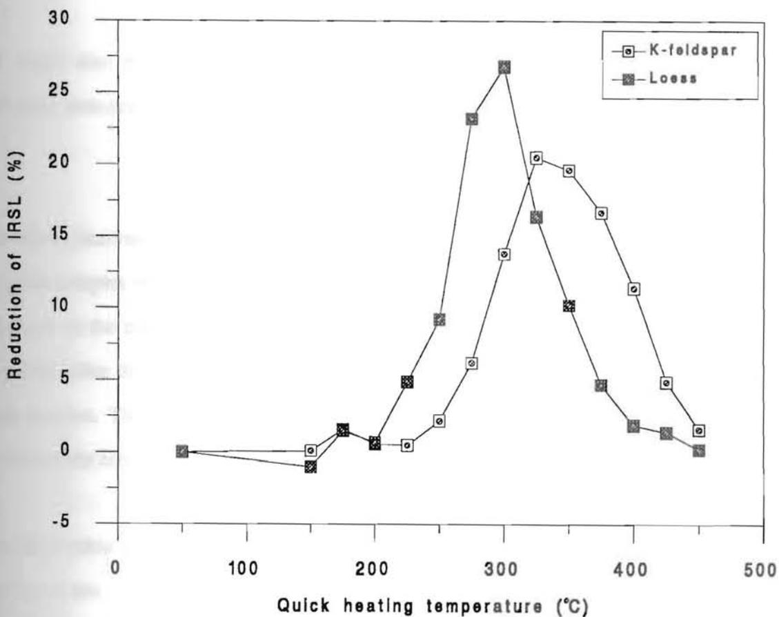
Figure 2.4.2. Quick heating curves of natural IRSL signals from loess and separated K-feldspar. (a) presented as the percent of the initial IRSL signal remaining (b) presented in form of IRSL signal reduction between each heating step. The loess sample is 88-12 from Luochuan, China. The K-feldspar is the separated fraction of sample (AF-3) from Natal, South Africa.
