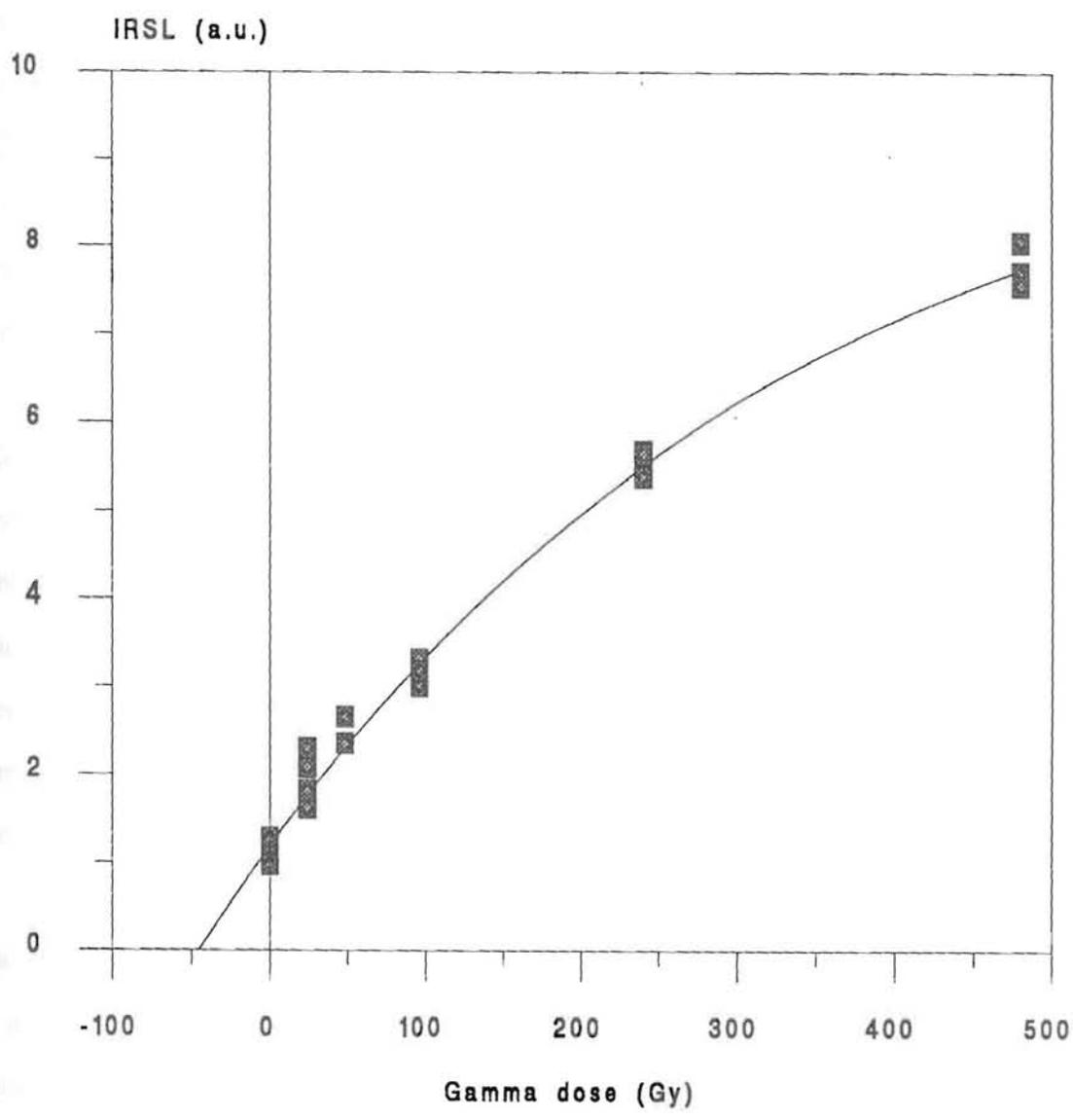
Fig. 4.2.2. IRSL from pellets of a sample as a result of  $\gamma$  irradiation. The sample is from the top of Rocourt loess section.
