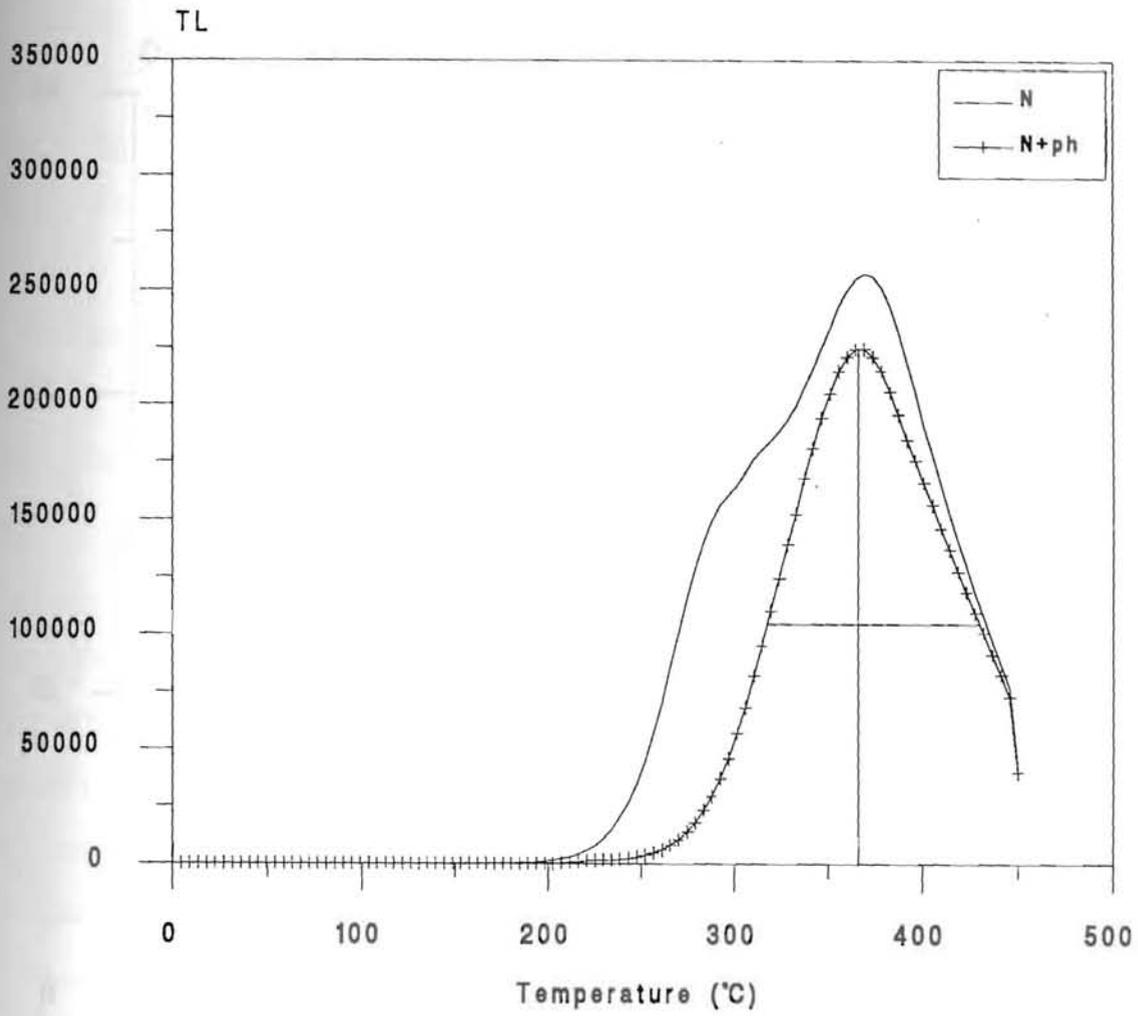
Figure 3.5.7. TL glow curves of sample Z29. The curves are natural and natural plus preheating for 10 minutes at 220°C.
