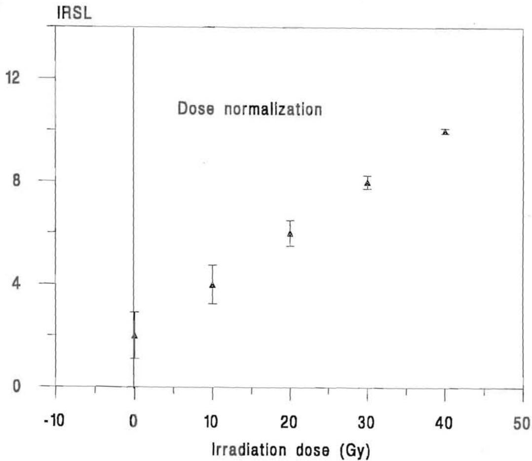
Figure 6.3.2. Schematic diagram showing the trend of disc-to-disc scatter for a insufficiently bleached sample after normalization procedures. (a) natural normalization (b) dose normalization.
