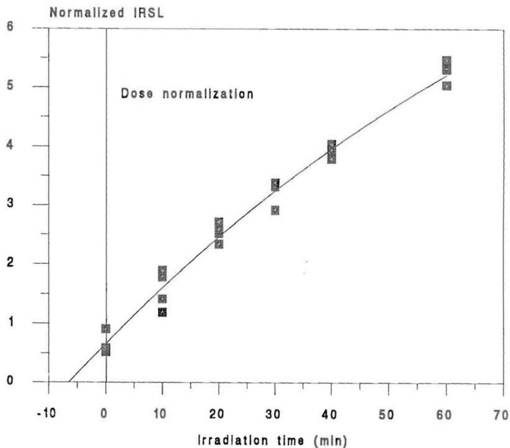
Figure 6.3.3. Disc-to-disc scatter shown for the additive growth curves of the K-feldspar fraction of sample AF-4 after normalization. (a) natural normalization (b) dose normalization (using response after a long bleach).
