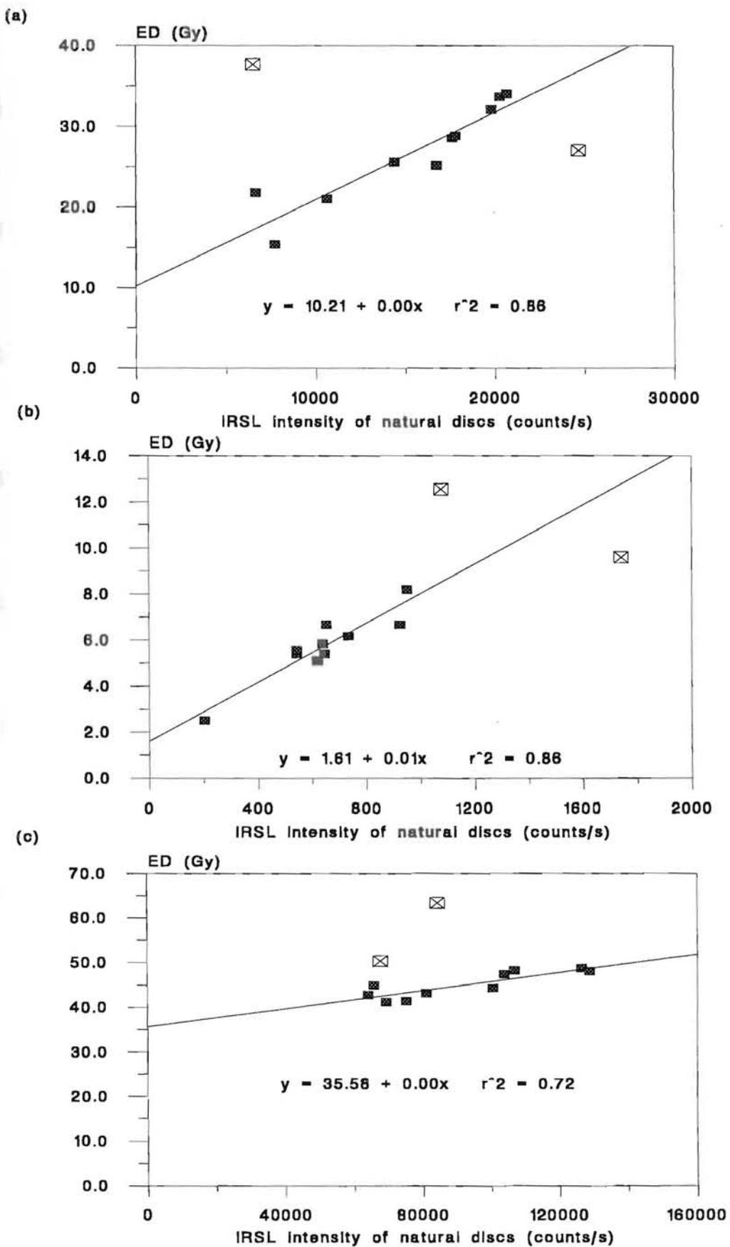
Figure 6.4.5. ED- $I_n$  plot showing a linear relationship for partially bleached colluvial samples. (a) AF-4, (b) STP-13 and (c) HIT-2. Data points were selected to meet the criterion of a correlation coefficient greater than 0.80. (⊗) Rejected discs (■) discs used for the fitting.
