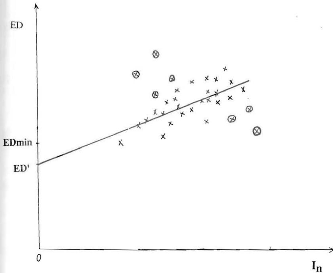
Figure 6.4.4. Schematic diagram showing the ED- $I_n$  plot method as used for the ED determination of an insufficiently bleached sample.
