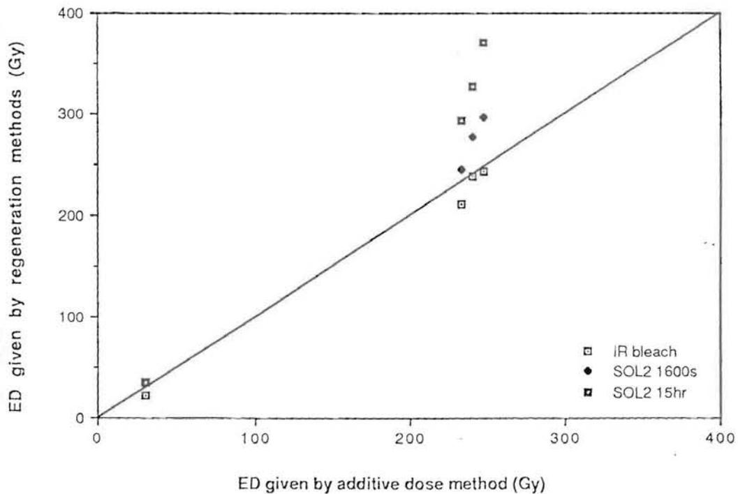
Figure 5.2.2. a) Sensitivity of initial IRSL signal measured after bleaching versus the initial sensitivity as obtained by extrapolation for the additive growth data sets. b) IRSL EDs obtained by the regeneration method using different bleachings versus that obtained by the additive dose method for 4 colluvial sediments. The line has a slope of 1.
