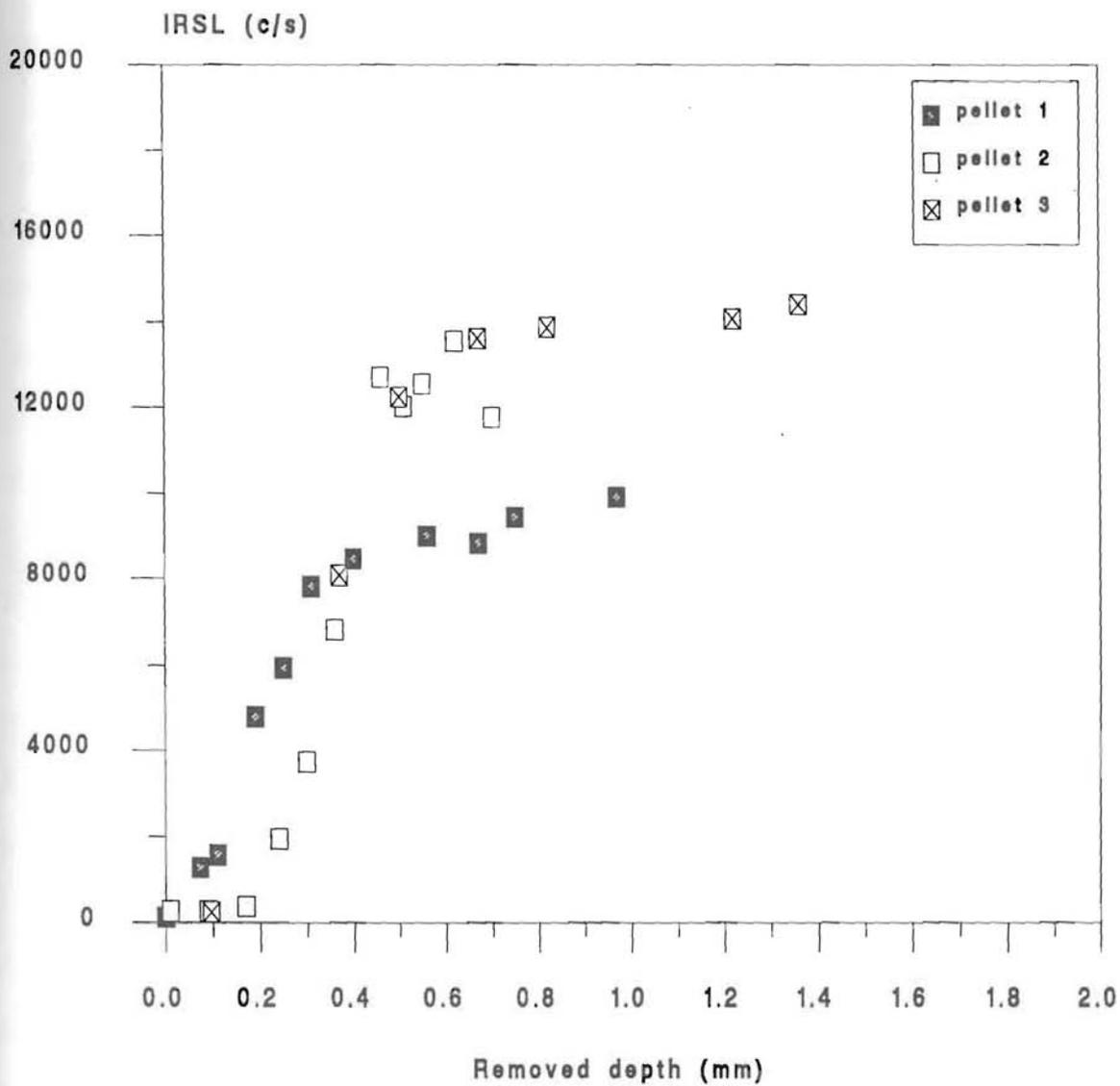
Fig. 4.4.6. Recovered IRSL signal as result of removing bleached grains.
