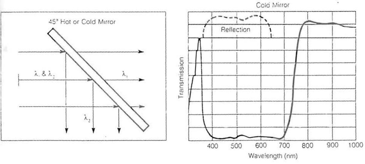
Fig. 4.3.2. (a) Schematic diagram of the optical unit (b) Characteristics of the cold mirror (from Ealing Catalogue )
