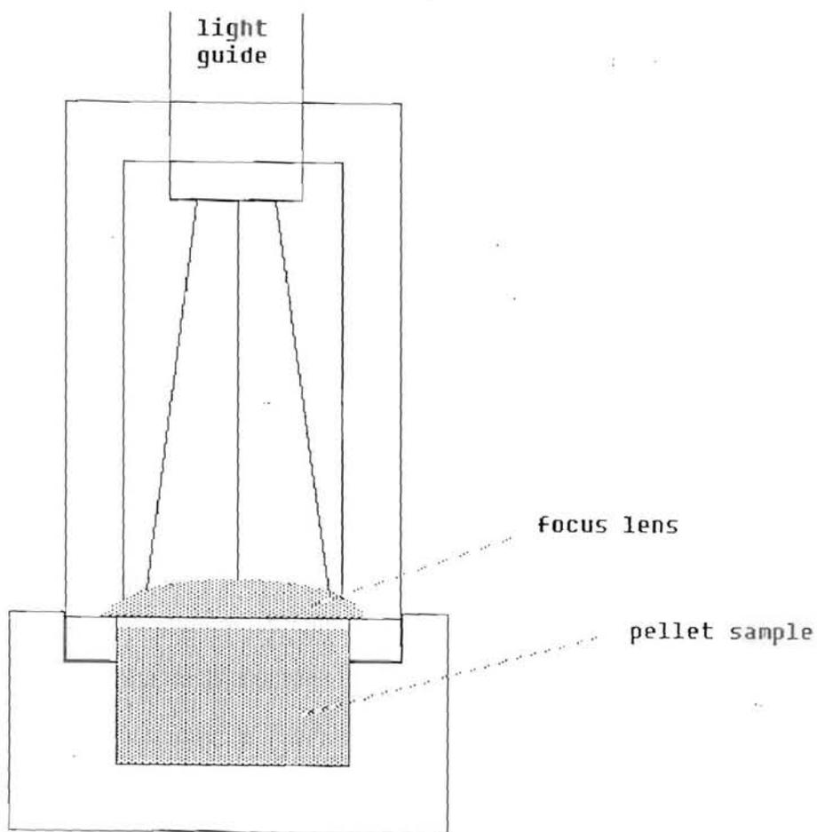
Fig. 4.3.3. Schematic diagram of the detector unit.
