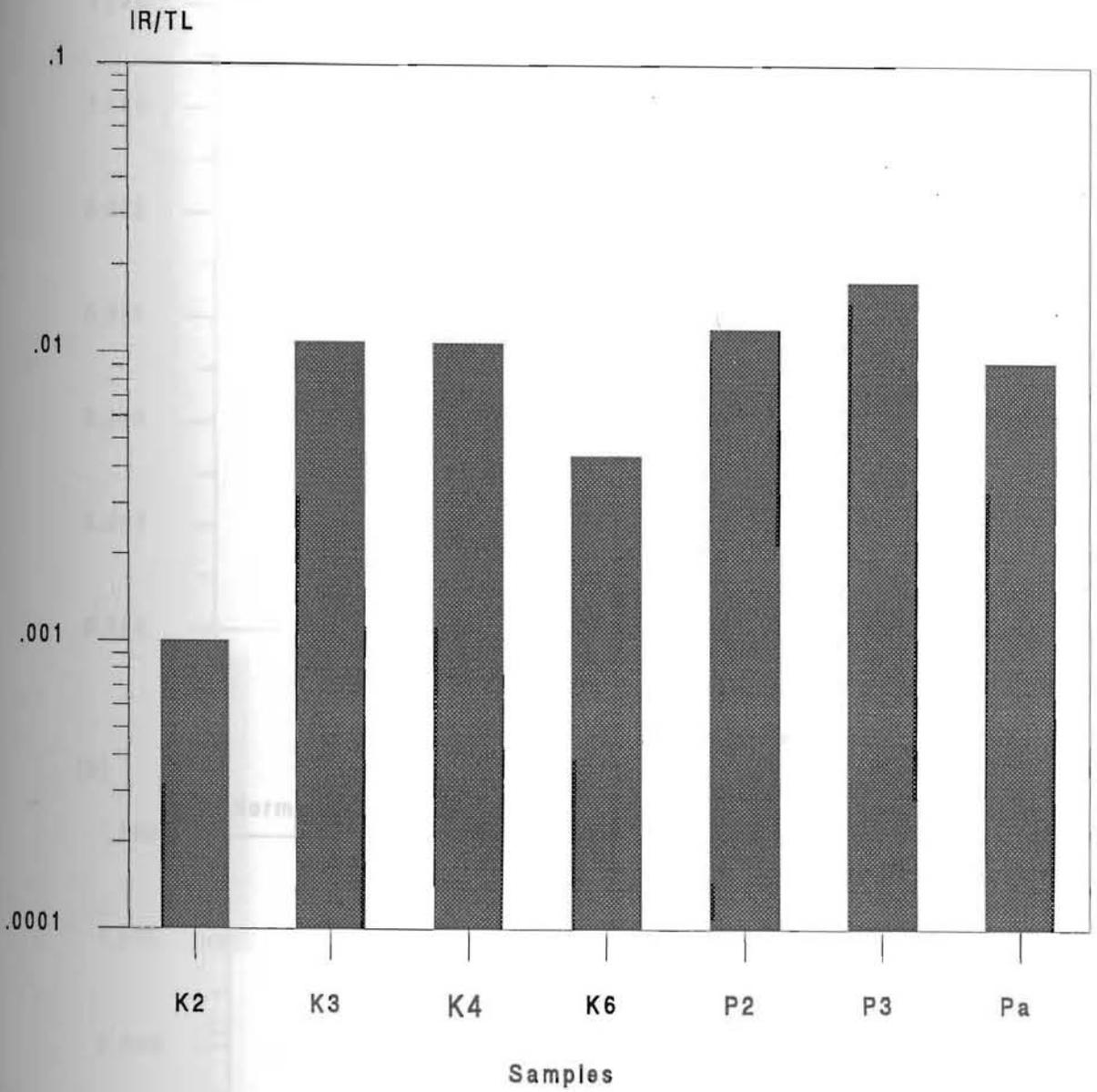
Figure 3.2.9. Ratio of IRSL from 1 second IR exposure and TL signal integrated from 20 to 450°C. Samples were preheated for 17 hours at 140°C after 12 Gy  $\beta$  irradiation.
