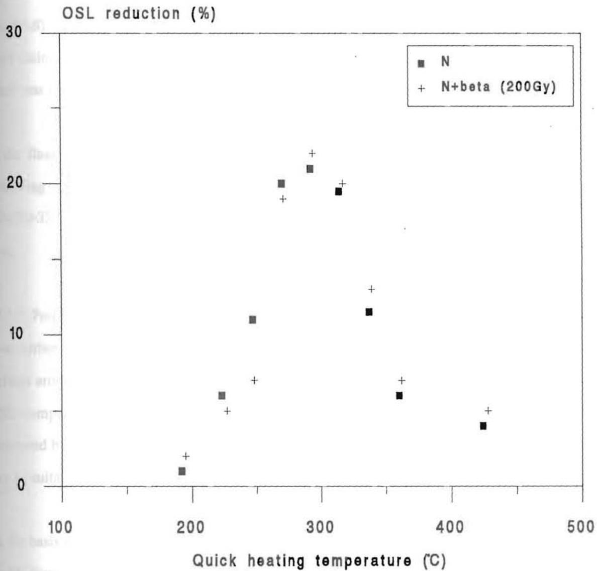
Figure 3.5.8. OSL reduction (%) by quick heating, after preheating 10 minutes at 210°C for natural and N+β aliquots for sample Z29.
