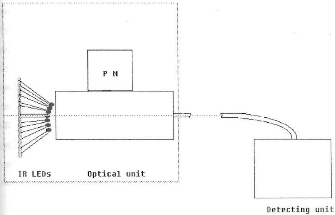
Fig. 4.3.1. Schematic diagram of the portable IR system.
