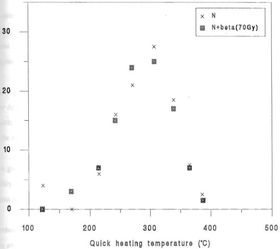
Figure 3.5.5. OSL reduction (%) by quick heating, after preheating a half hour at 160°C for natural and N+β dosed discs from sample Z10.
