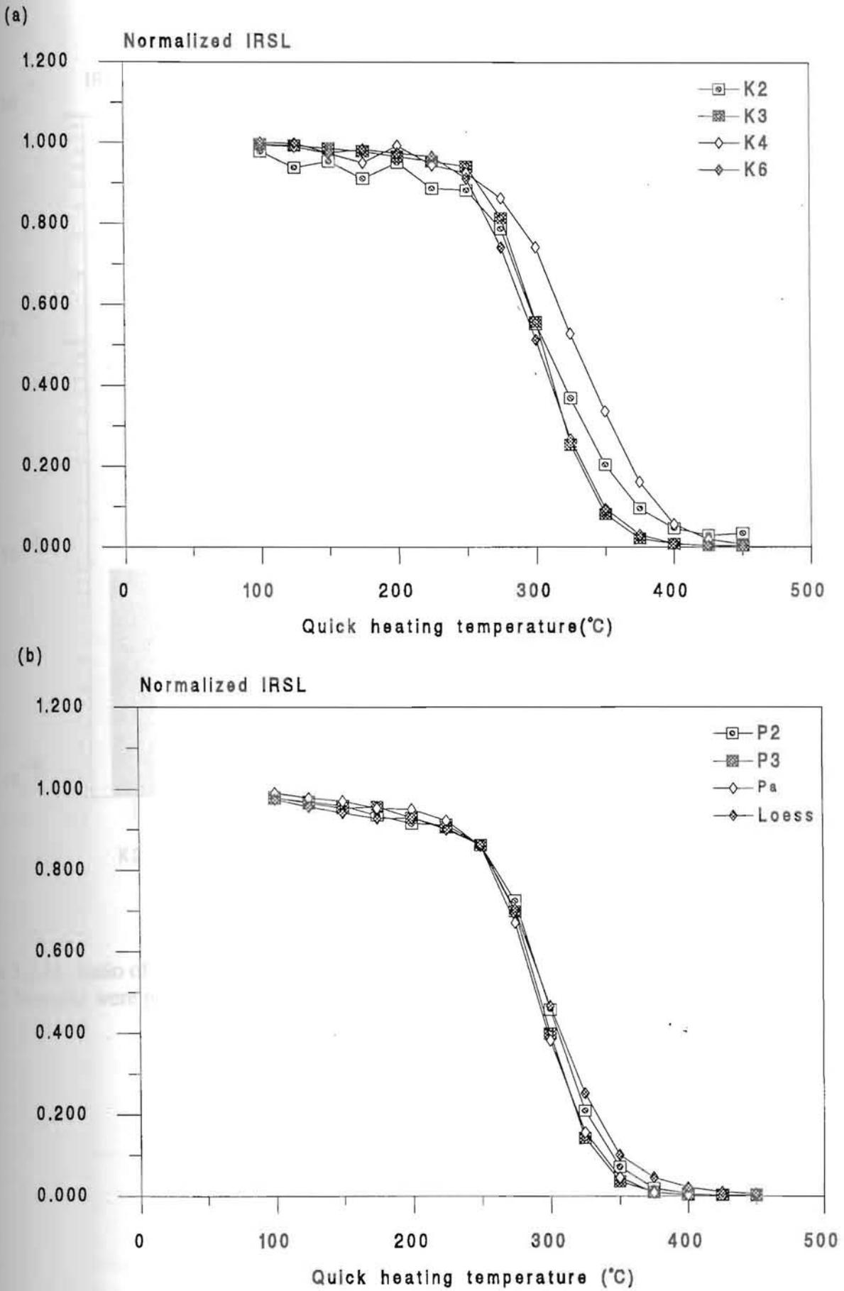
Figure 3.2.10. Quick heating of feldspar samples after 17 hours preheating at 140°C (see text). (a) K-feldspar samples (b) plagioclase feldspar samples.
