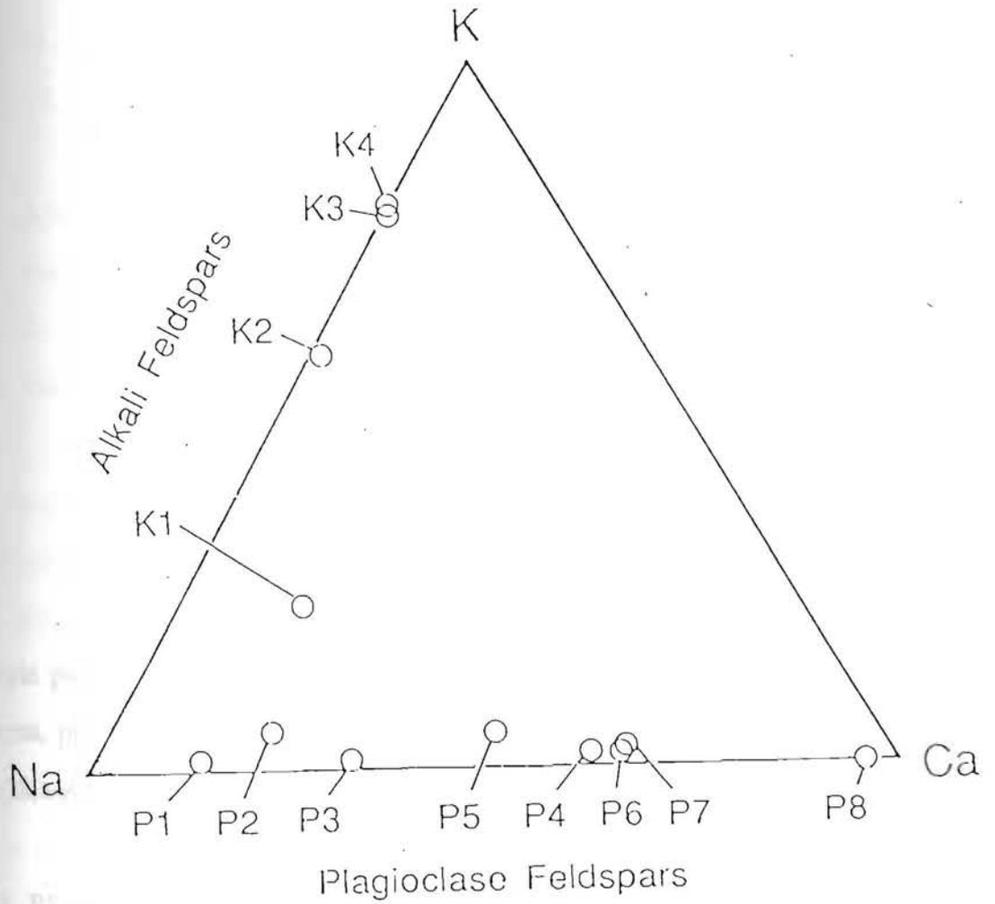
Figure 3.2.1. The feldspar ternary diagram showing the composition of fourteen feldspar minerals used in this study (from Huntley et al. 1988).
