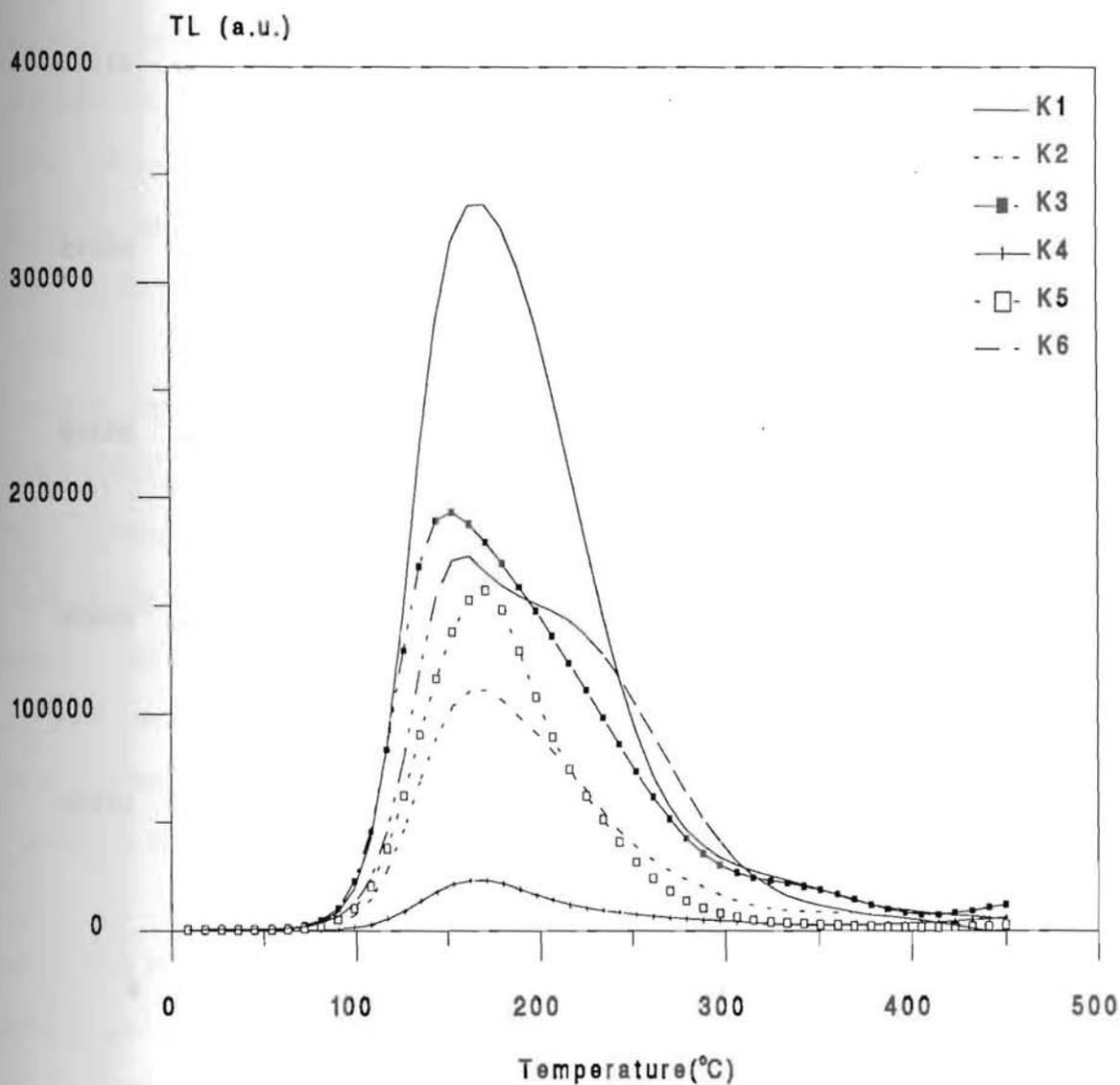
Figure 3.2.2. TL glow curves of K-feldspars. TL measurement took place with less than one hour delay after  $\beta$  irradiation (12 Gy).
