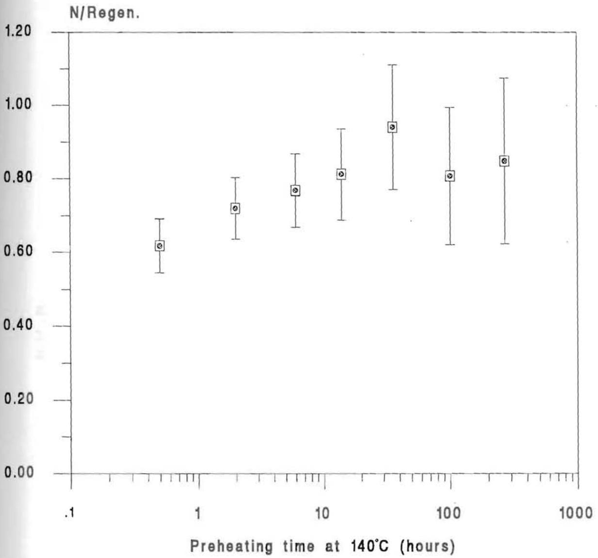
Figure 3.5.9. Preheating plateau of IRSL signals from natural and  $\beta$  dosed (74 Gy) loess discs. Sample was QTL89D (ED 51 Gy) from Rocourt, Belgium. Preheating was at 140°C.
