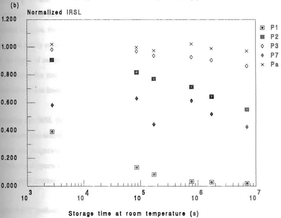
Figure 3.2.6. Decay of IRSL at room temperature. (a) K-feldspar samples (b) plagioclase feldspar samples. Samples were not preheated after irradiation. Each signal was normalized to the first measurement (see text). Each point is the mean of four aliquots.
