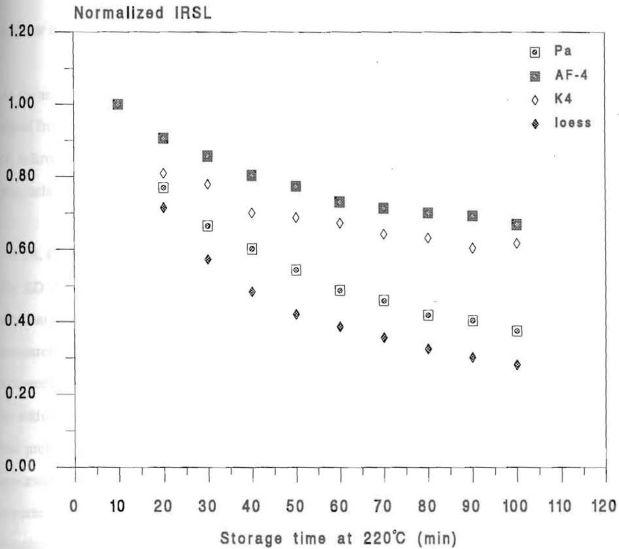
Figure 3.4.2. Comparison of the thermal stability of the IRSL signal from a K-feldspar extract and loess and the pure mineral samples (Pa and K4) used in the previous section (3.3.).
