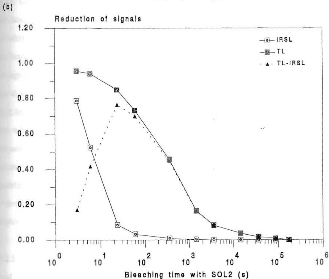
Figure 6.2.4. Bleaching of the TL and IRSL signals of K-feldspar fraction of sample NEW-3. The TL was measured after IRSL measurement with 1 second IR exposure. (a) reduction of signals (b) fractional reduction of bleachable signals and the difference (TL-IRSL) between the signals after the same bleaching. Signals after 48 hours bleaching were used as the unbleachable components and subtracted from the total signals.
