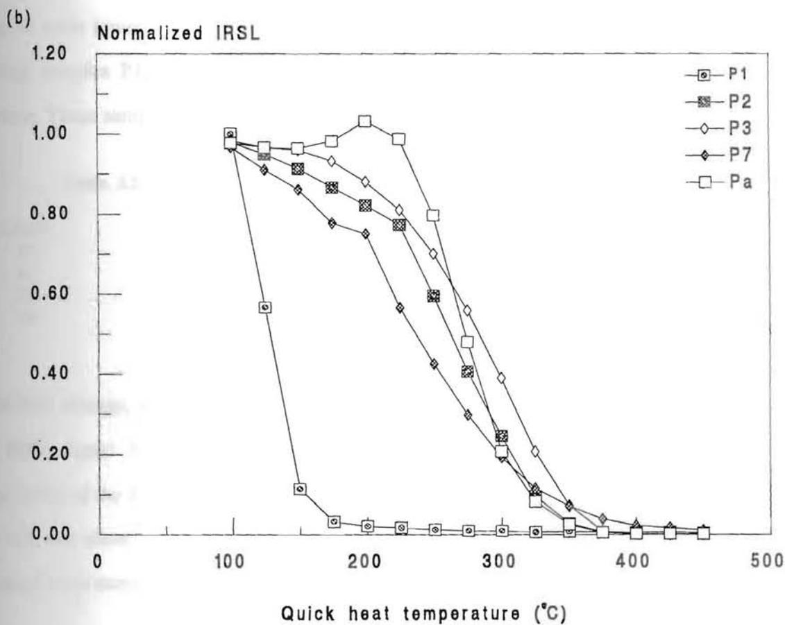
Figure 3.2.7. Quick heating of feldspar samples after  $\beta$  irradiation. (a) K-feldspar samples (b) plagioclase feldspar samples. Discs were heated at  $5^\circ\text{C/s}$  to the temperature shown and cooled to  $50^\circ\text{C}$ . IRSL was measured at  $50^\circ\text{C}$  with a 0.1 second IR exposure.
