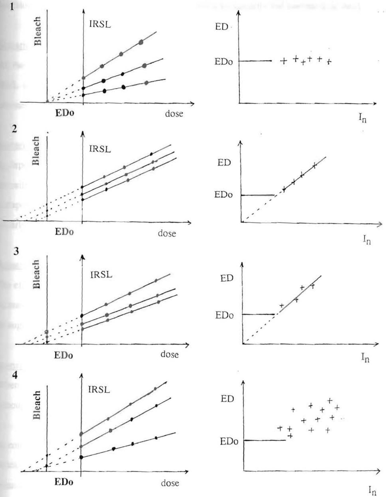
Figure 6.4.3. Possible connections between ED and  $I_n$  for different conditions of deposition.
