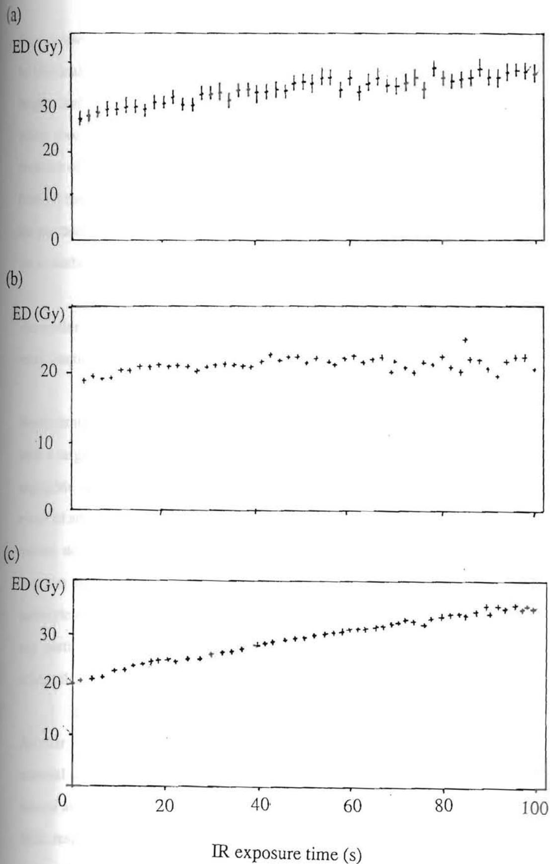
Figure 6.3.1. Shine plateau for sample AF-4. (a) fine grain disc1 (b) fine grain disc2 (c) coarse grain (125-150 $\mu$ m) K-feldspar disc. Single disc regeneration method was used.
