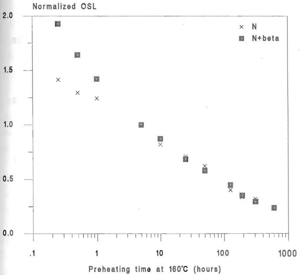
Figure 3.5.4. Isothermal decay curves for OSL signal of sample Z10 at 160°C. Samples were N and N+beta , with a  $\beta$  dose 70 Gy. Normalization was for the data points for 5 hour storage.
