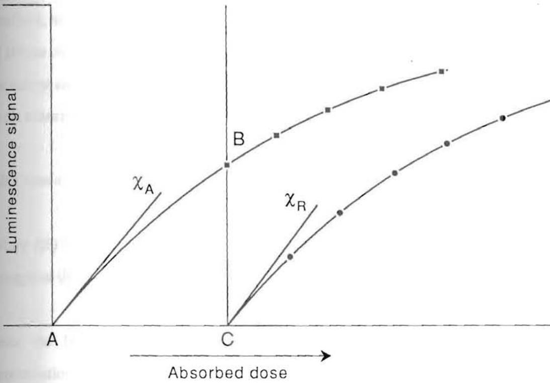
Figure 5.3.1. Schematic diagram of luminescence signal growth curves: the response to added dose (■) and response to dose after laboratory bleaching (●).
