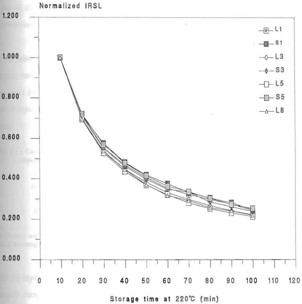
Figure 3.3.6. Effect of 220°C storage for natural loess and palaeosol samples from Luochuan section. The loess (palaeosol) samples are distinguished by L an S prefixes.
