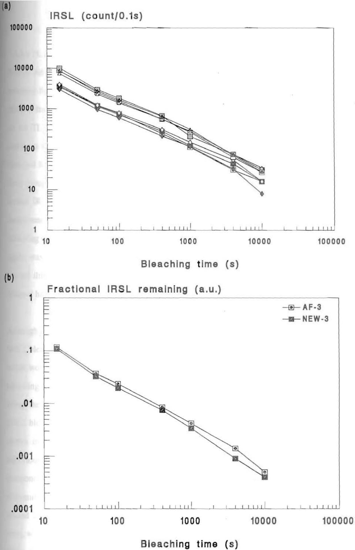
Figure 6.2.3. Bleaching of the IRSL by the SOL2 of two samples of different initial levels. (a) unnormalized discs (b) after natural normalization (each point is the average of six discs).
