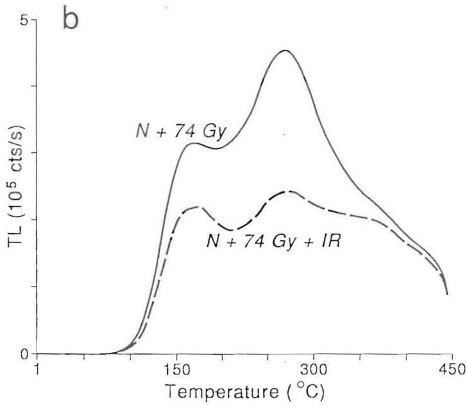
3.3.7. TL glowcurves using Corning 5-60+HA3 ( $5^{\circ}\text{C/s}$ ) for loess from Rocourt, Belgium showing the effect of 1000 second IR exposure. (a) natural; (b) natural plus 74 Gy  $\beta$  dose.
