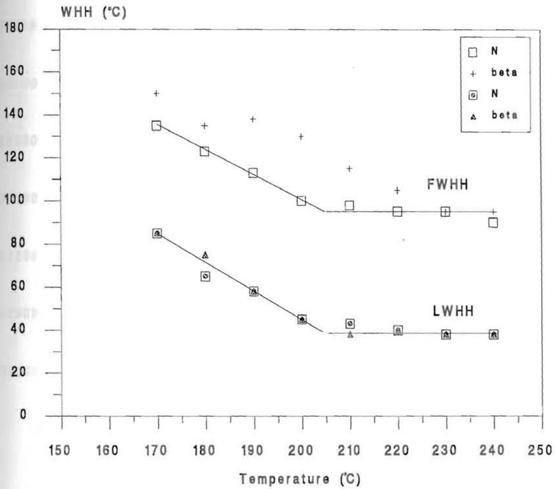
Figure 3.5.6. Plot of FWHH (see text) of TL glow curve versus preheating temperature for ten minutes. The left part of the WHH gives a better result. Results shown for Natural and second glow TL.
