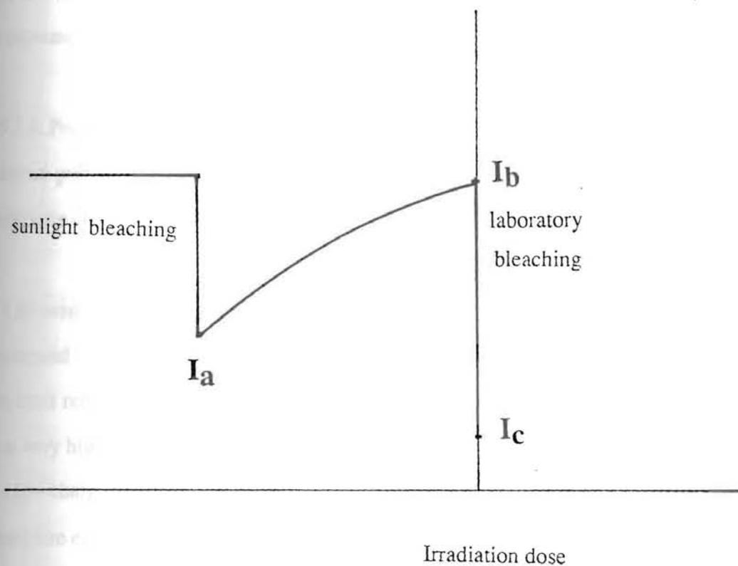
Figure. 5.3.2. Schematic diagram showing the change in concentration of H type (the hard to bleach) trapped charges as a result of natural and laboratory bleaching procedures.
