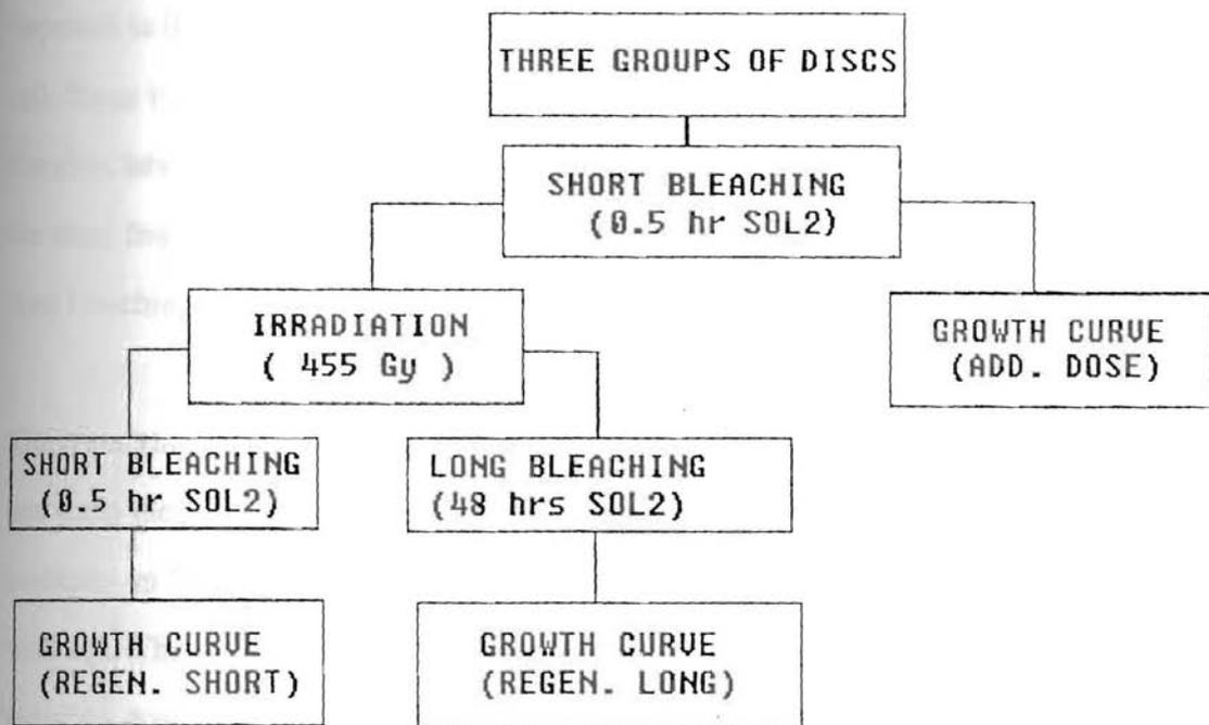
Figure 5.4.1. Experimental sequence for the "artificial colluvial sediment"
