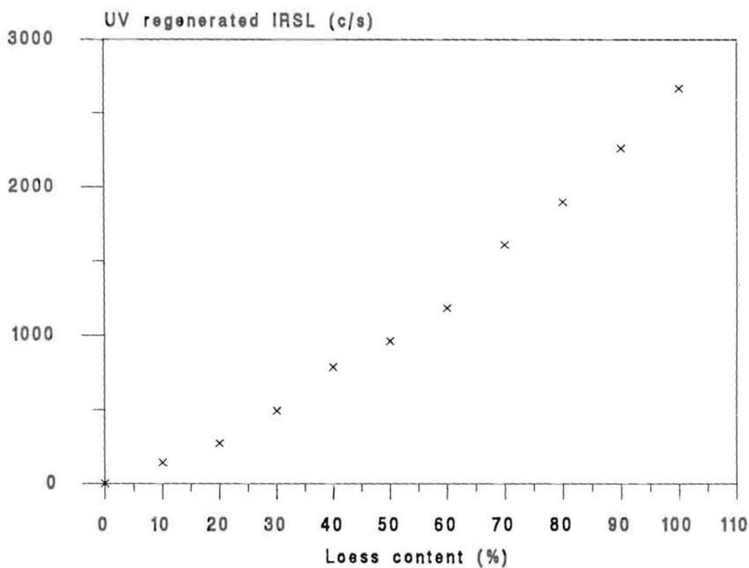
Fig. 4.4.2. IRSL signals of pellets of mixed loess and carbonate. (a) natural signal (b) u.v. regenerated signal after bleaching with visible light.
