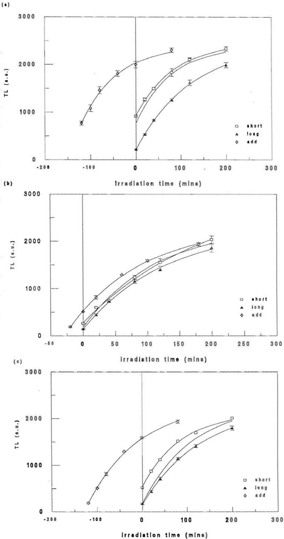
Figure. 5.4.4. TL growth curves. (a) colluvial sediment (b) young aeolian sediment (c) old aeolian sediment. Sample discs are the same as the IRSL in Fig.5.4.4. The dose rate was 3.79 Gy/min.
