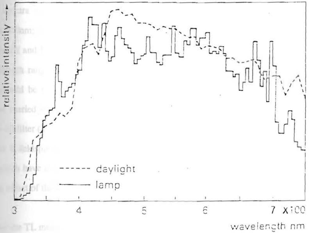
Figure 2.3.1. Spectrum of the SOL2 solar simulator (from the company brochure).
