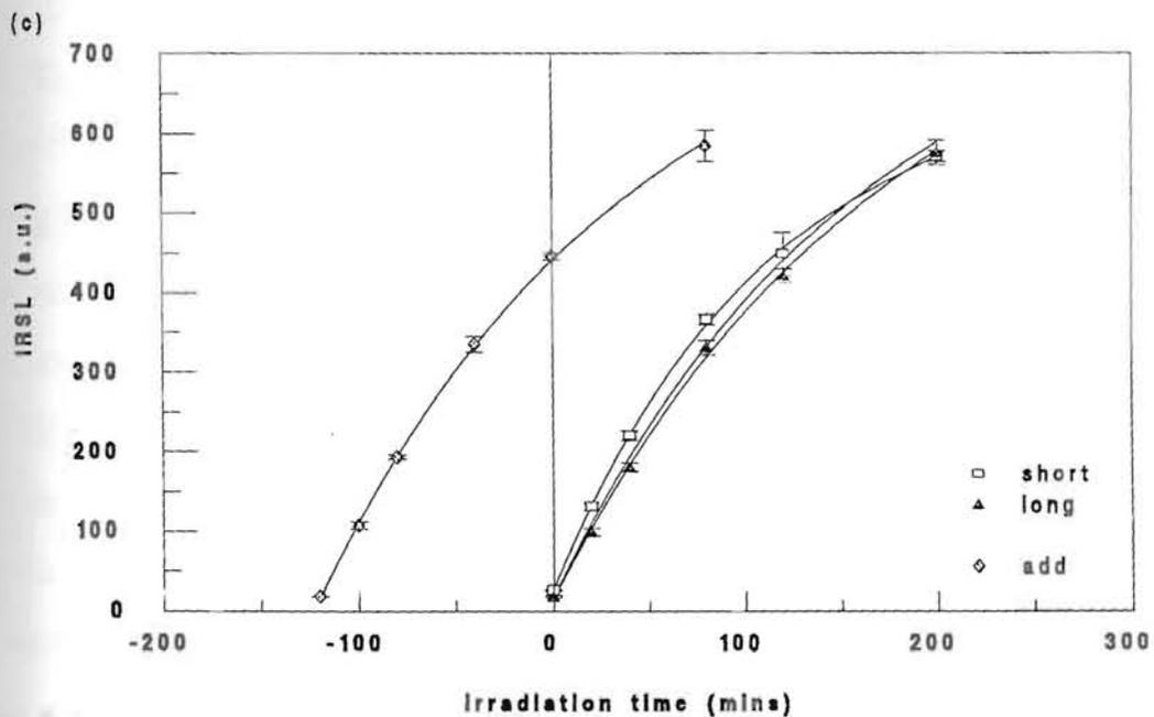
Figure 5.4.3. IRSL growth curves. (a) Colluvial sediment (b) young aeolian sediment (c) old aeolian sediment. The dose rate was 3.79 Gy/min.
