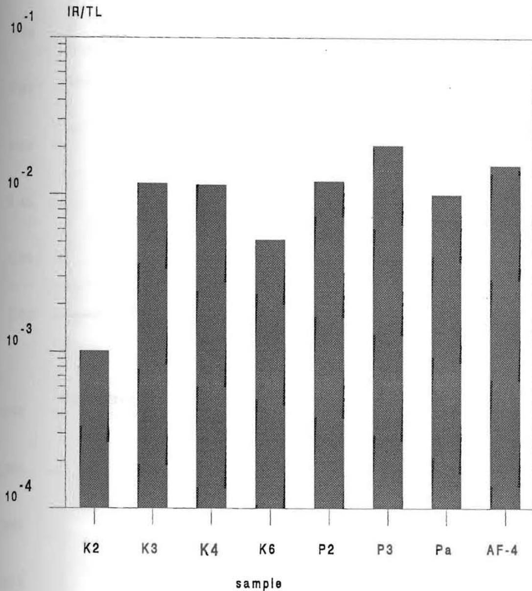
Figure 3.2.11. Ratio of IRSL from 1 second IR exposure and TL signal integrated from 20 to 450°C. Samples were preheated for 10 minutes at 220°C after 12Gy  $\beta$  irradiation.
