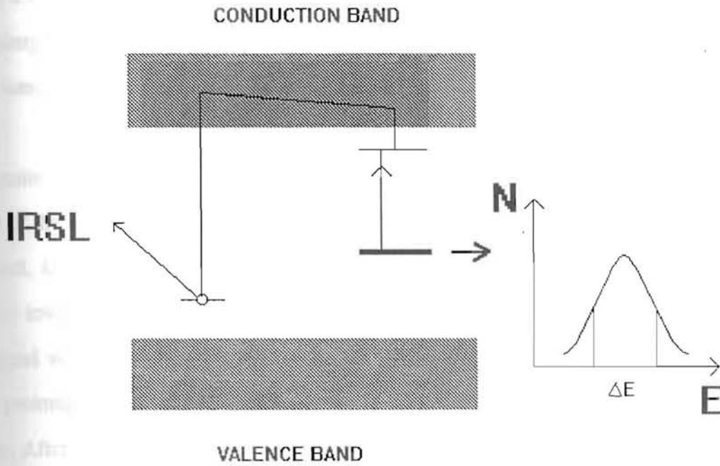
Figure 3.2.14. Diagram of IR stimulation process. The activation energy has a continuous distribution in energy range  $\Delta E$ .
