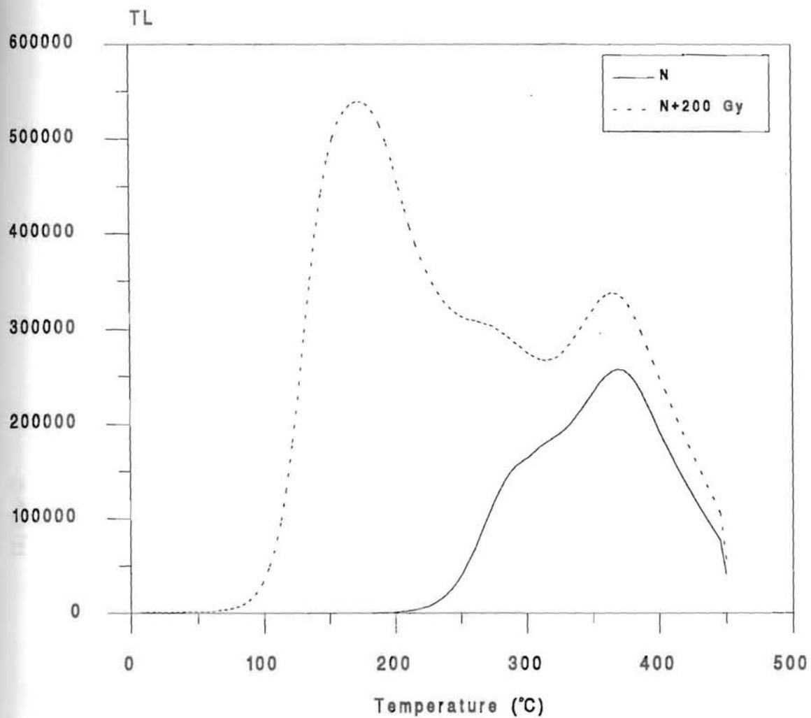
Figure 3.5.2. Typical TL glow curves of samples Z29. (a) Natural + 200Gy  $\beta$  dose; (b) Natural.
