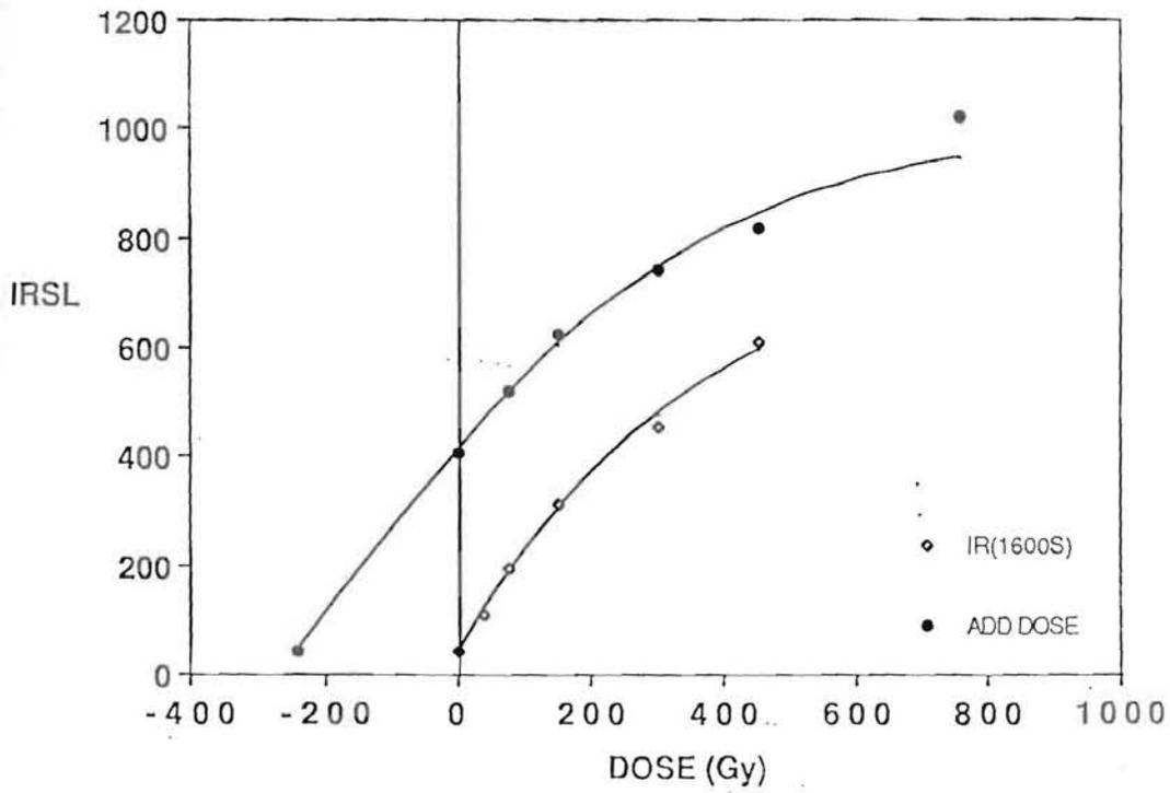
Figure 5.2.1. Growth curves for sample AF-1. a) Regeneration after exposure to IR and SOL2. b) additive dose and regeneration after IR bleaching.
