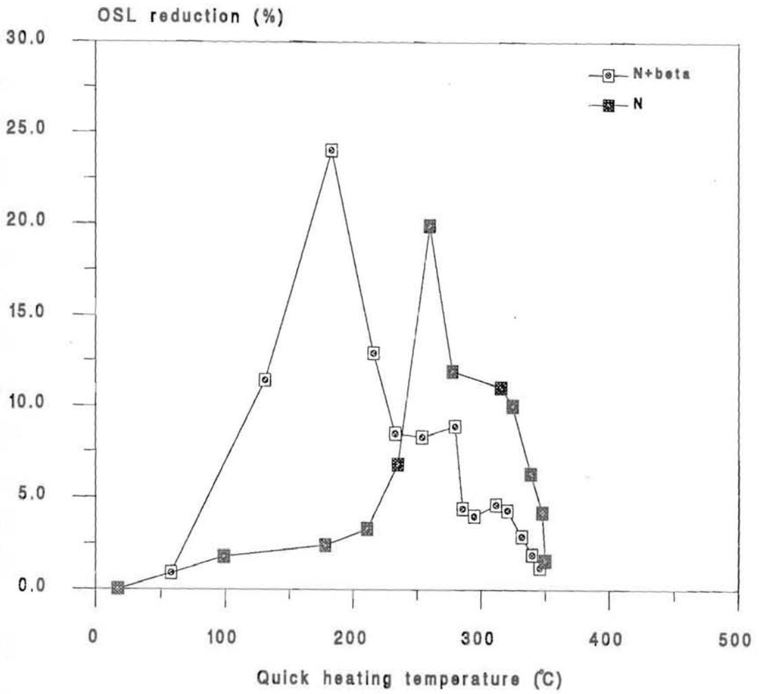
Figure 3.5.1. Quick heating of OSL signal from natural and natural plus  $\beta$  dose (200 Gy) discs of sample Z29.
