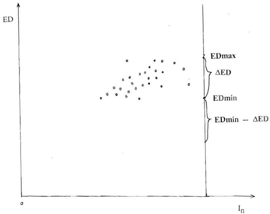
Figure 6.4.7. Schematic diagram showing method 2. The most likely value for  $ED_0$  is given by the minimum ED and the range ( $\Delta ED$ ) of the ED obtained.
