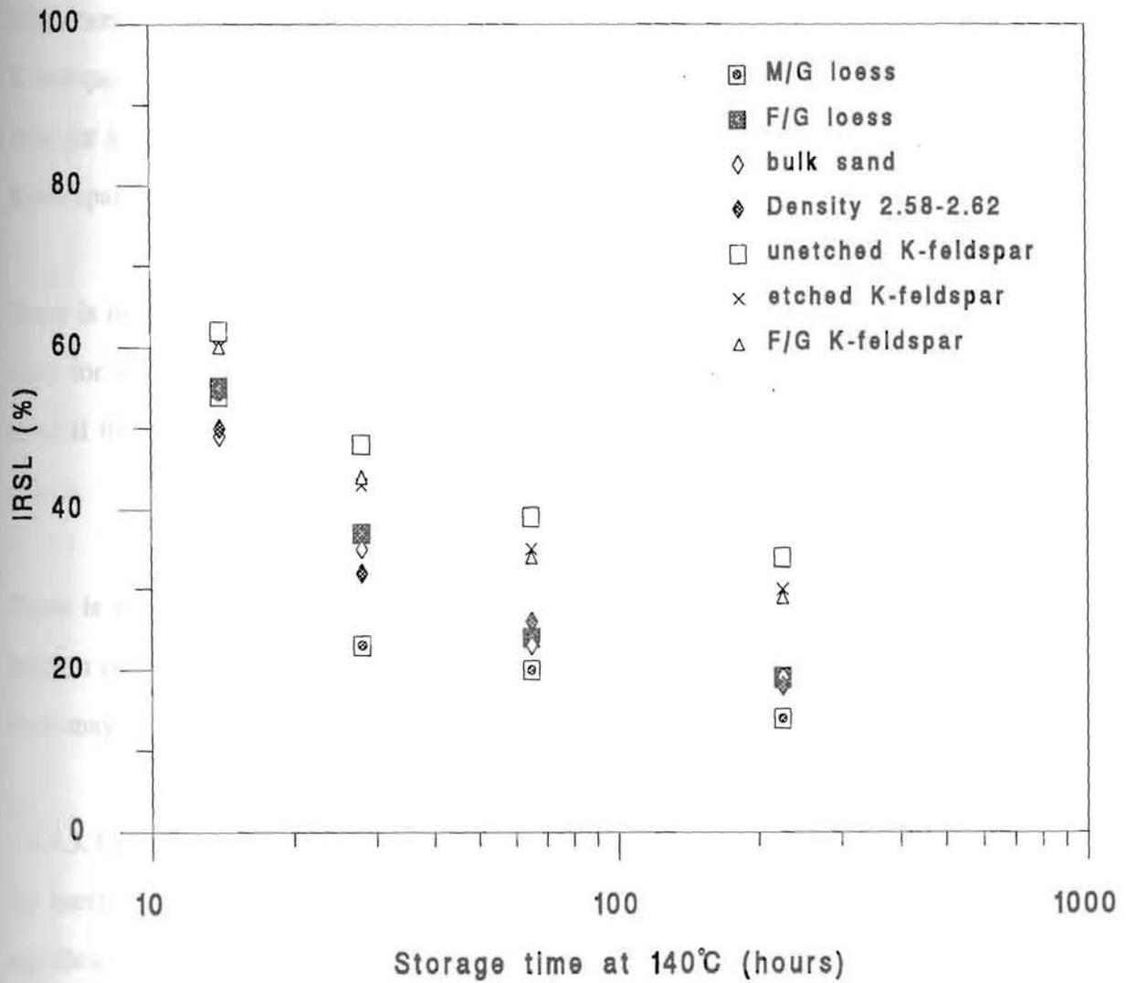
Figure 3.4.1. Comparison of the thermal stability of the IRSL signal from different mineral components of New Zealand sand and Chinese loess with different grain size fractions (as detailed in text). Samples were given five hours bleach with SOL2 solar simulator followed by a 100 Gy  $\beta$  dose.
