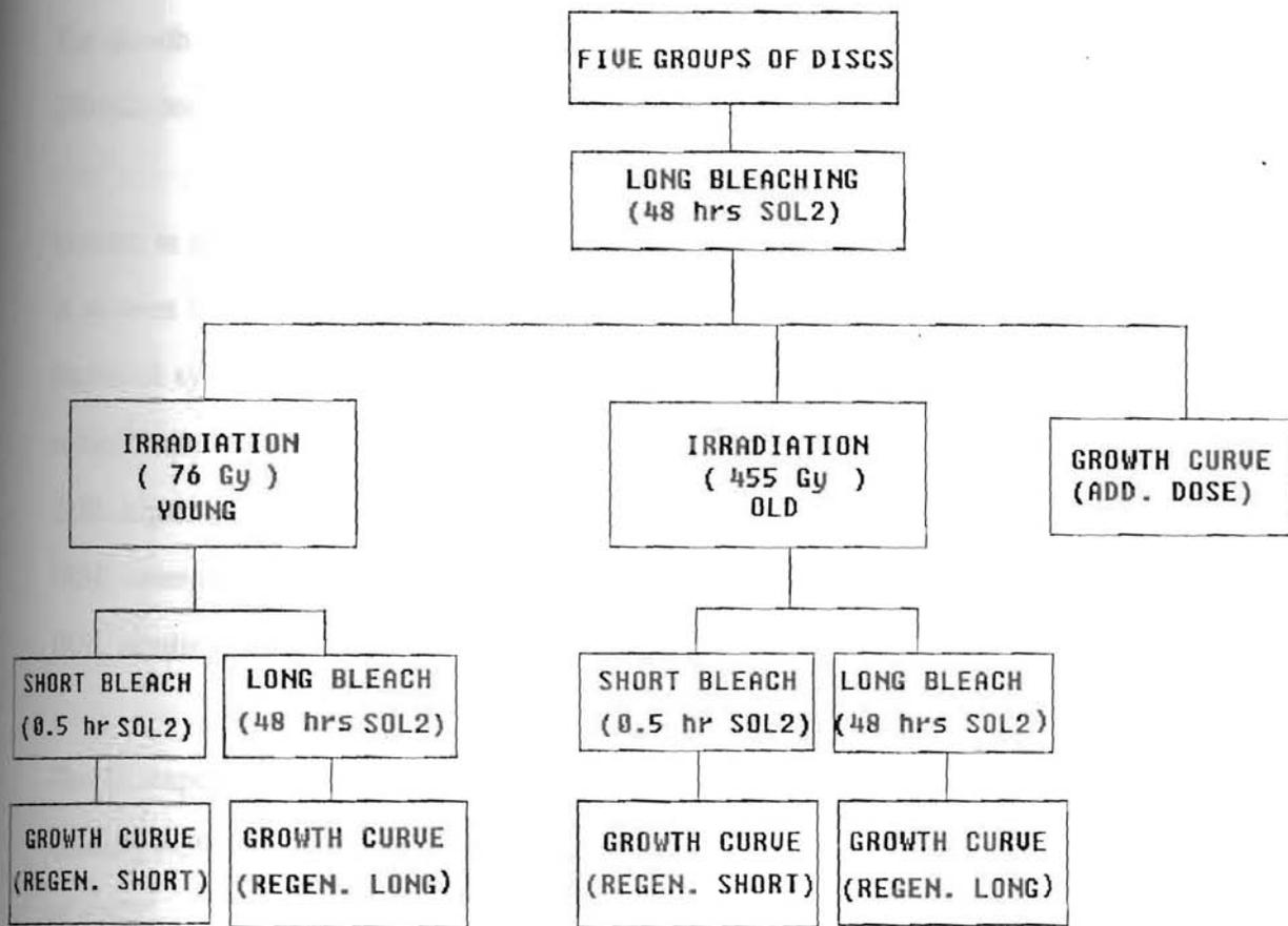
Figure. 5.4.2. Experimental sequence for the "artificial aeolian sediment"
