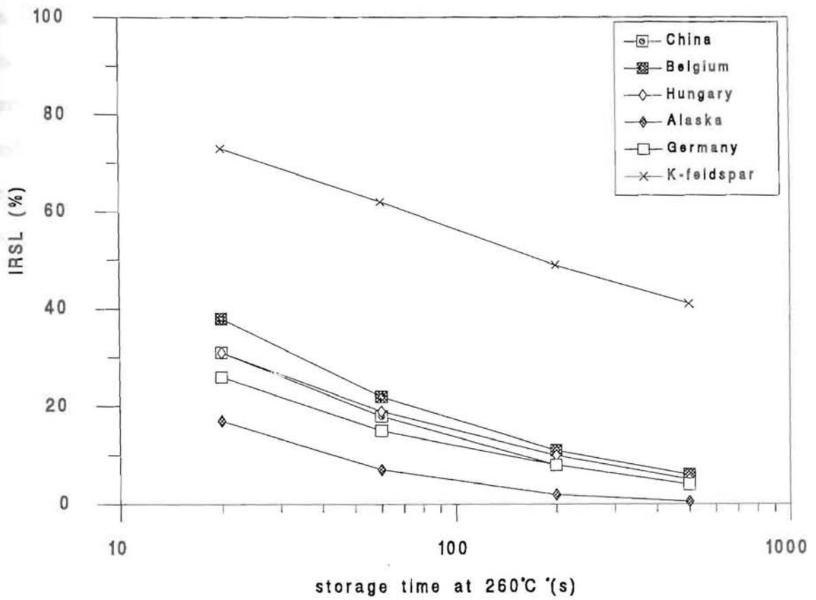
Figure 3.3.4. Loess and K-feldspar (Z29) natural discs stored at (a) 230°C and (b) 260°C.
