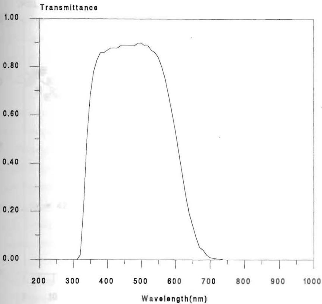
Figure 2.3.2. Spectral response of the BG39 filter (from the Schott catalogue).
