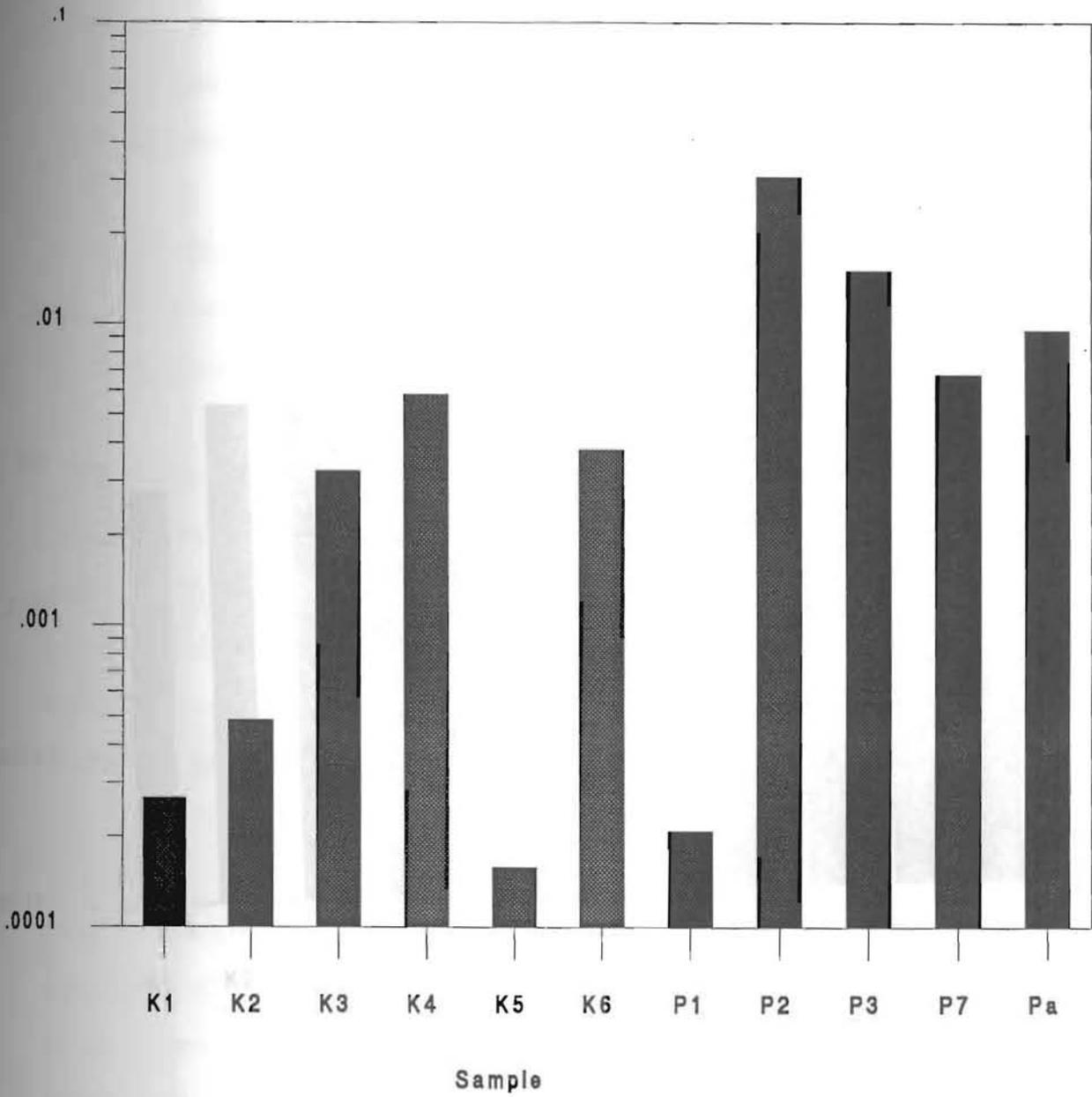
Figure 3.2.4. Ratio of beta induced IRSL from 1 second IR exposure and the TL signal integrated from 20 to 450°C for different feldspar samples.
