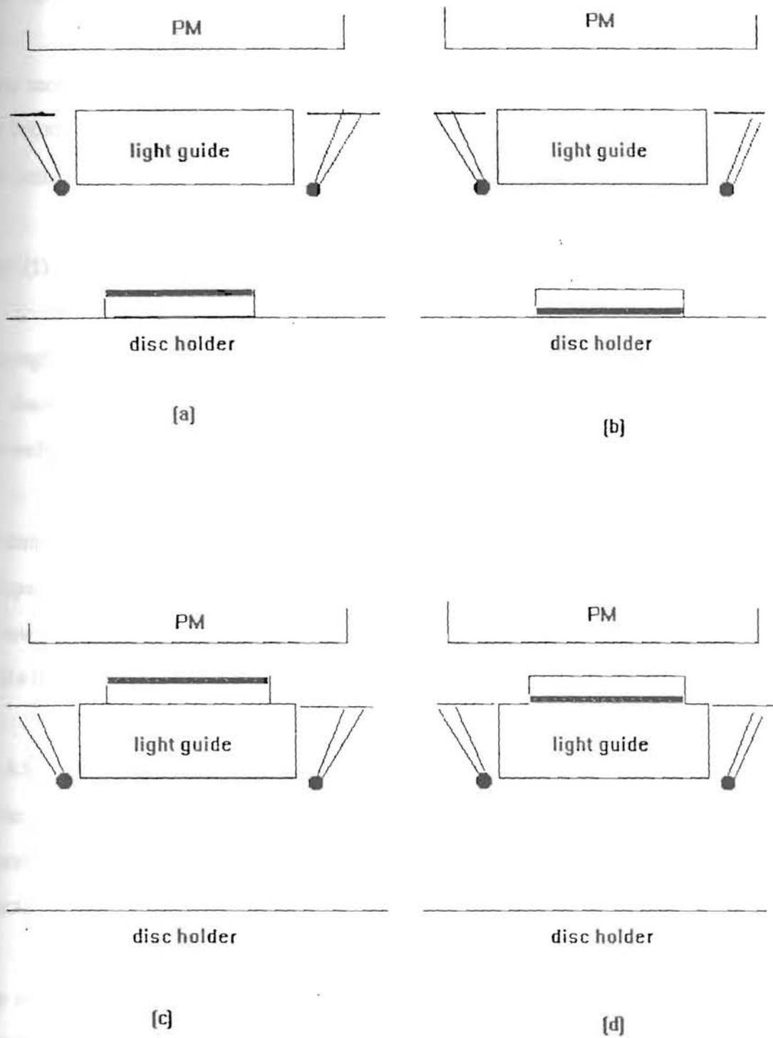
Fig. 4.4.5. Schematic diagram showing the positions of feldspar chip during measurements.
