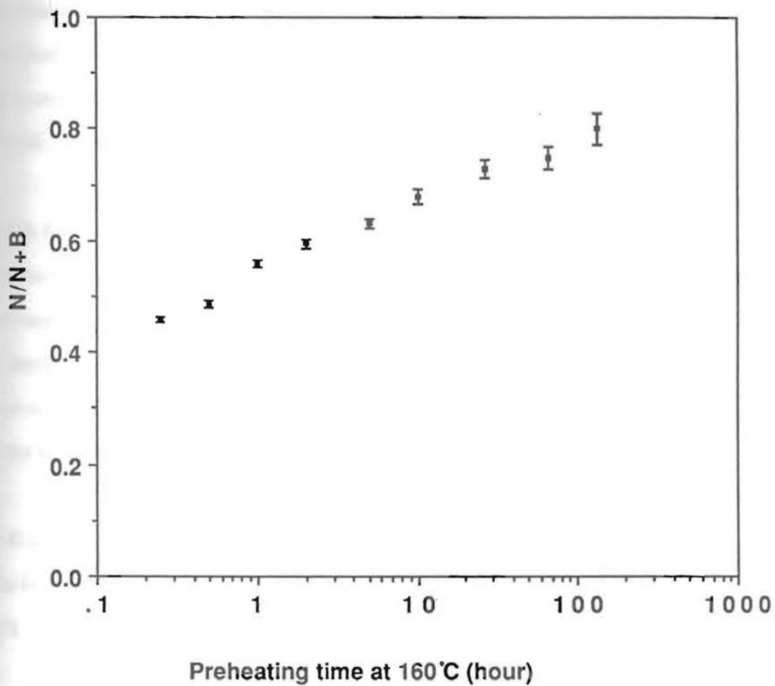
Figure 3.5.10. Preheating plateau of OSL signal for loess sample 88-12 (ED 215 Gy) from Luochuan, China. Preheating was at 160°C. The added beta dose was 200 Gy.
