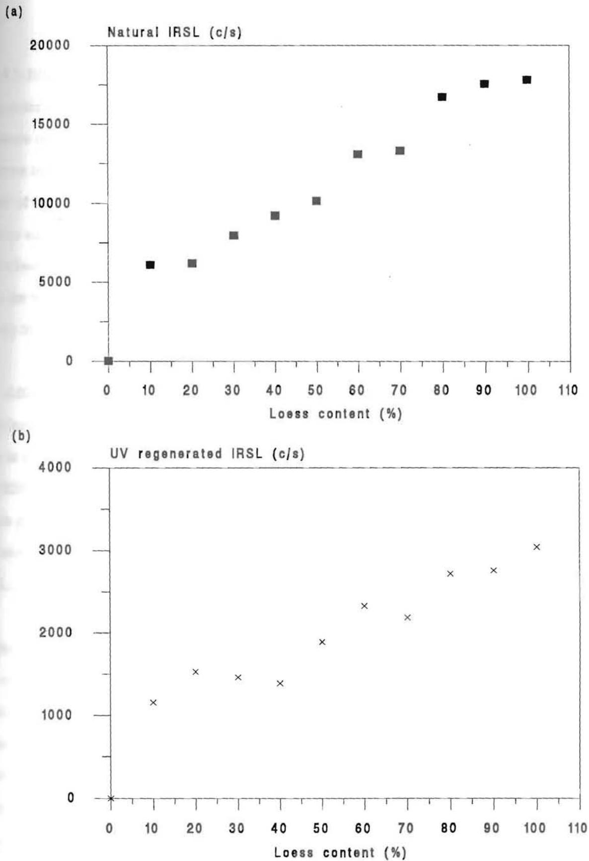
Fig. 4.4.3. IRSL signals of pellets of mixed loess and quartz crystals. (a) natural signal (b) u.v. regenerated signal after bleaching with visible light.
