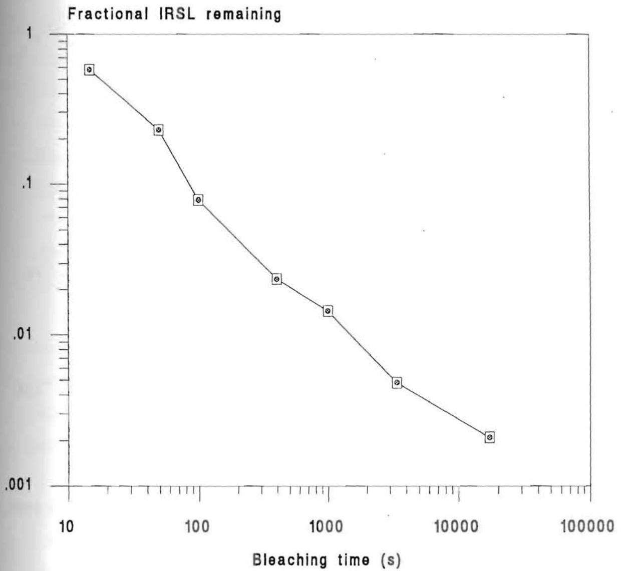
Figure 6.2.1. IRSL bleaching with sunlight on a clear day in Aberystwyth. The air temperature was  $4 \pm 3^\circ\text{C}$ .
