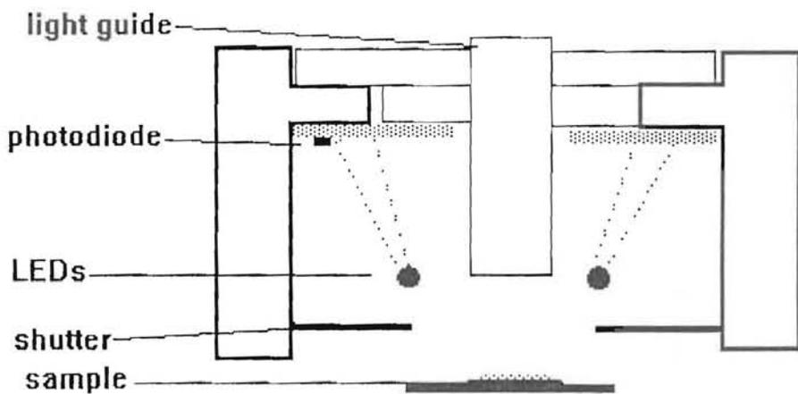
Figure 2.1.1. Schematic diagram shows the Manual Daybreak IRSL system built during this study.
