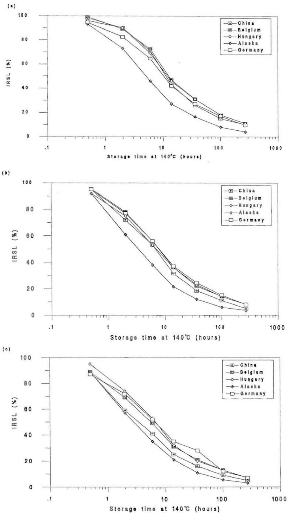
Figure 3.3.2. Results for loess samples stored at 140°C. (a) natural; (b) natural plus  $\beta$  dose (74Gy); (c)  $\beta$  dose (74 Gy) regenerated signal.
