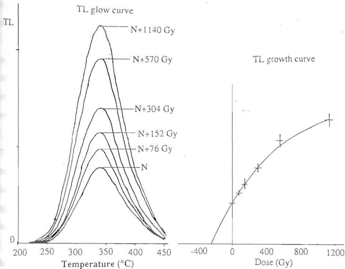
Figure 7.3.1. TL glow curves and growth curve of sample NEW-2. (a) glow curves (b) growth curve for 275-400°C. Glow curves were shifted to align the peaks at about 340°C.
