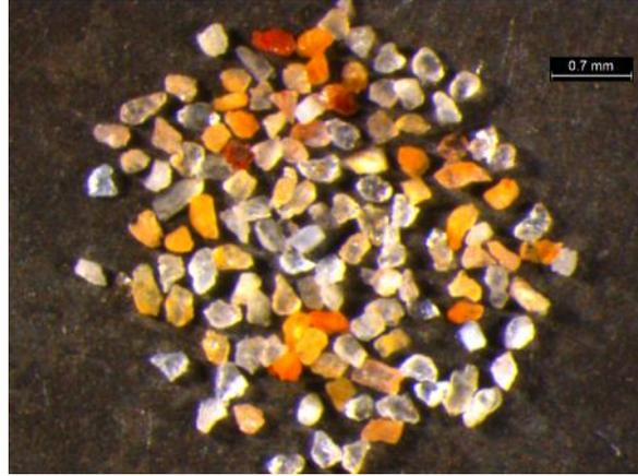
**Figure 4-2.** A K-rich feldspar aliquot from sample KHUT-1 containing a mixture of K-rich feldspar, quartz, plagioclase and possibly other minerals. Sodium polytungstate ( $<2.58 \text{ g/cm}^3$ ) was used to remove quartz, plagioclase and heavy minerals from the 180–212  $\mu\text{m}$  grain size fraction. The separate was then etched for 10 min with a diluted HF acid (10%) solution. The microphoto was taken using a digital camera mounted on a Leica MZ16A stereo microscope.
