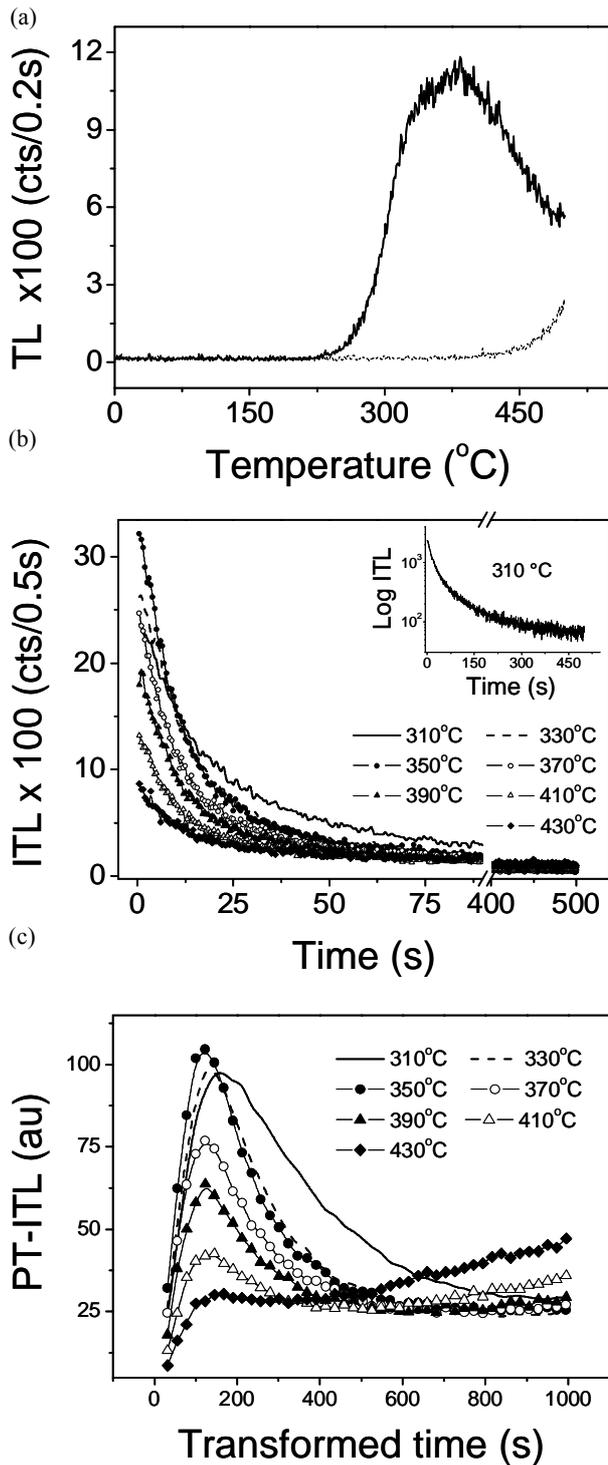
**Figure 3:** a) TL peak of an aliquot of quartz from a modern sample (BTh0) after a dose of 34 Gy and a preheat of 260°C for 10s. TL was measured at the rate of 5°C/s. The dotted curve is the repeat TL run after the TL signal had been measured. b) Natural isothermal TL decay curves measured at different temperatures c) same data plotted as peak transformed isothermal TL (PT-ITL) curves.
