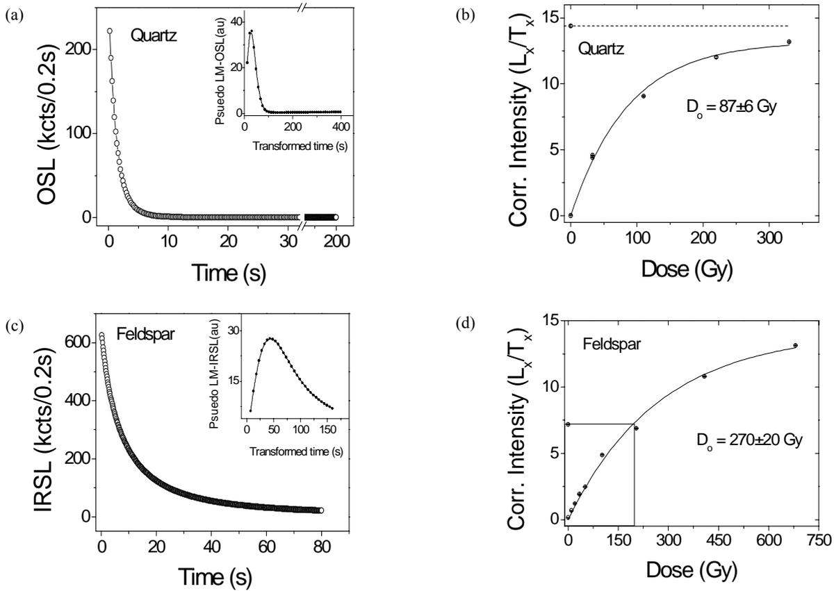
**Figure 1:** a) Natural OSL decay curve from a quartz aliquot of sample K-IX/49. The inset shows a pseudo LM-OSL curve derived from the same data. b) Dose response curve for the same aliquot of quartz. c) Natural IRSL decay curve from a feldspar aliquot of sample K-IX/49. The inset shows a pseudo LM-IRSL curve. d) Dose response curve for the same feldspar aliquot. The first 0.8s was used for signal integration in both IRSL and OSL decay curves.
