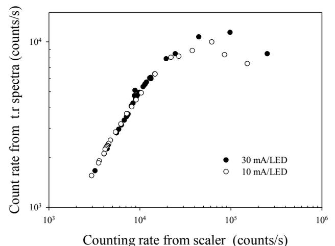
**Figure 4:** A comparison of counting rates obtained at 10 and 30 mA per LED.
