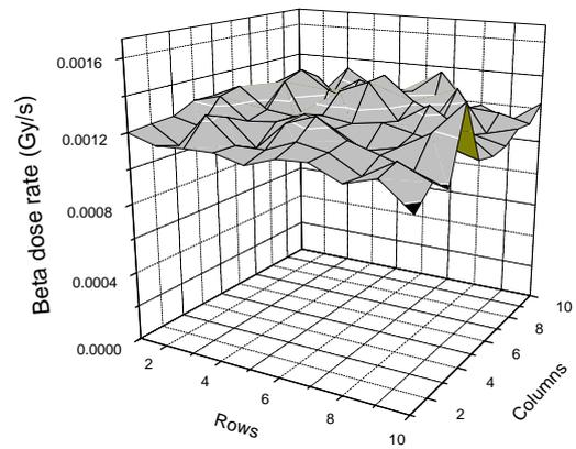
**Figure 2:** 3-D plot of dose rate ( $z$  axis) as a function of grain position ( $x, y$ ) on ten-by-ten grid position for source 5626 (24.1 MBq SIF ceramic source).
