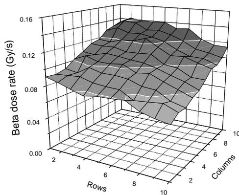
**Figure 3:** 3-D plot of dose rate ( $z$  axis) as a function of grain position ( $x, y$ ) on ten-by-ten grid position for source 6100 (1.48 GBq SIF ceramic source).
