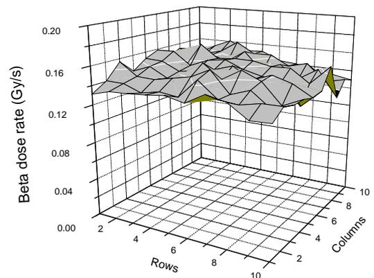
**Figure 4:** 3-D plot of dose rate ( $z$  axis) as a function of grain position ( $x, y$ ) on ten-by-ten grid position for source 6088 (1.48 GBq SIF ceramic source).
