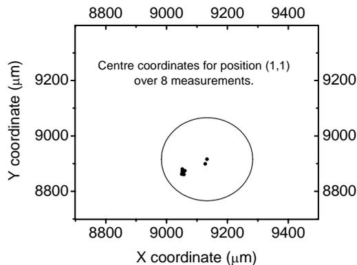
**Figure 5:** Plot of centre co-ordinates for position (1, 1) as obtained over 8 OSL measurements made in a SAR cycle. Circle drawn to show size of hole with its centre at the first measurement position.
