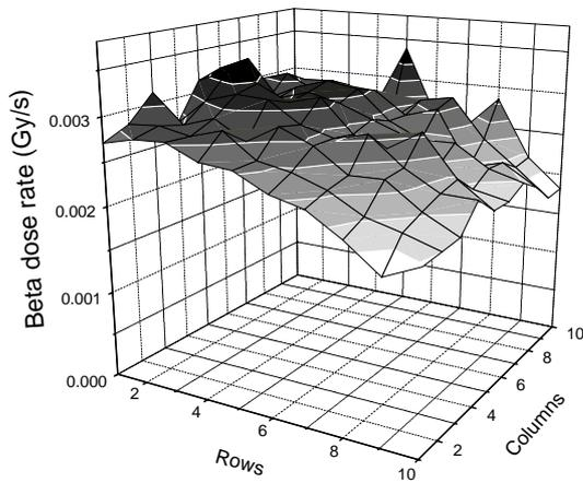
**Figure 1:** 3-D plot of dose rate ( $z$  axis) as a function of grain position ( $x, y$ ) on ten-by-ten grid position for source 5583 (74 MBq SIP silver plaque source).
