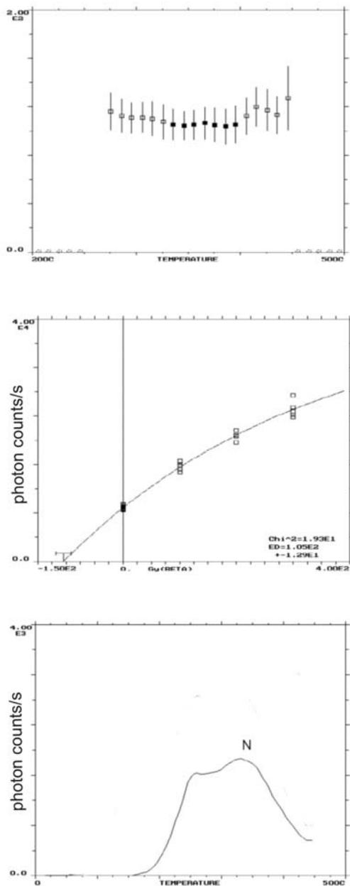
**Figure 1:**  $D_e$  plateau test (top), TL growth curve 300-360°C (middle, saturating exponential fit, not corrected for anomalous fading) and two NTL glow-curves of #1 Ulmener Maar (bottom).
