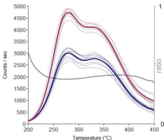
**Figure 7:** TL glow-curves of sample 5 (Devonian siltstone). Upper curves (thick line: mean) NTL after 150°C preheat for 19 h only (T). Lower curves: (thick line: mean) NTL after 150°C preheat for 19 h and simultaneous 1 GPa pressure (P+T). Grey line: ratio of (P+T)/T.
