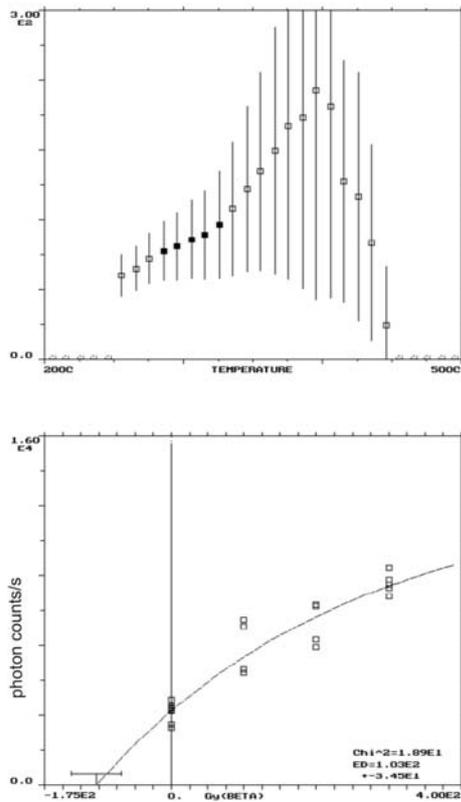
**Figure 5:**  $D_e$  plateau test and TL growth curve of #2 Pulvermaar, 125-250 μm, 280-320°C (saturating exponential fit), not corrected for anomalous fading.
