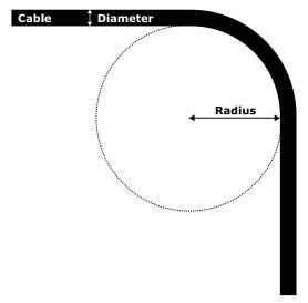
Figure 3: Cable Bend Radius
