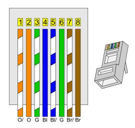
Figure 7: Pin and Pair Assignment of TIA-568-B
