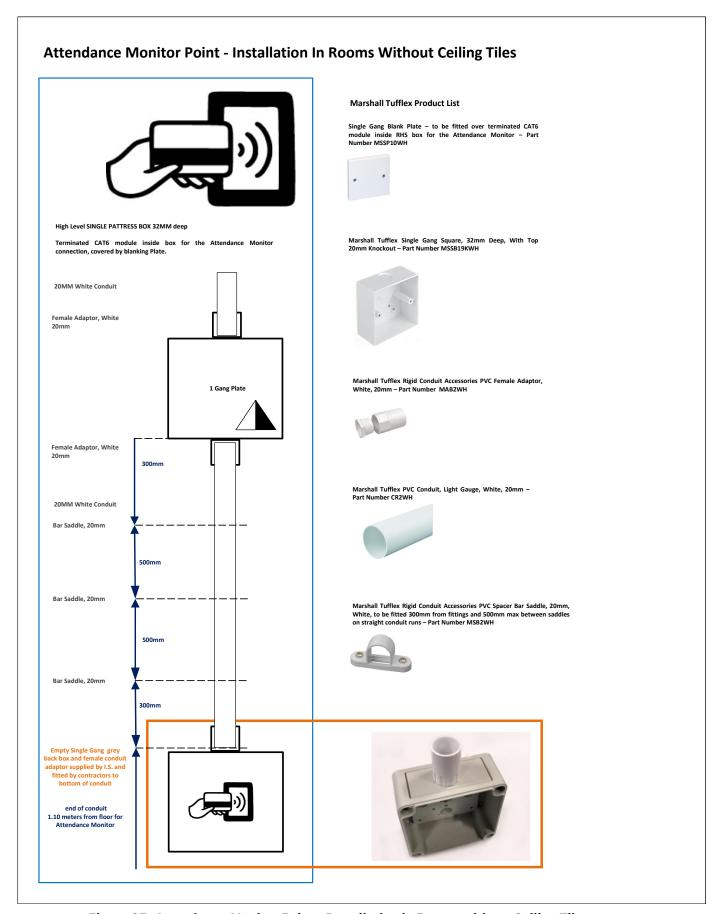
Figure 25: Attendance Monitor Point - Installation in Rooms without Ceiling Tiles
