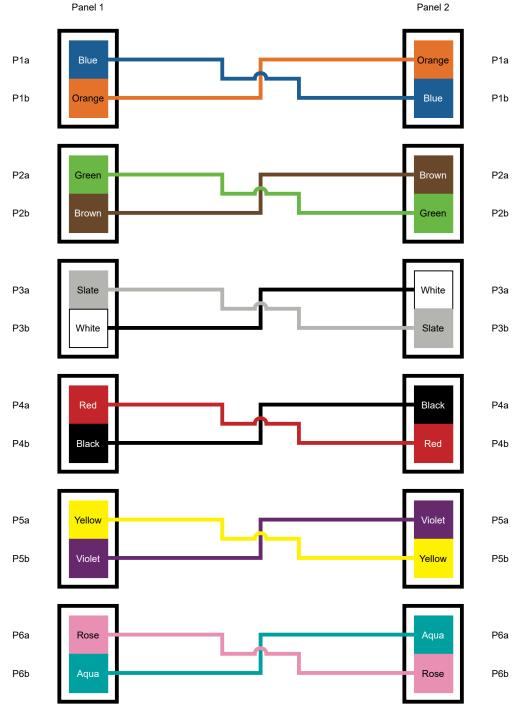
Figure 23: Fibre-Optic Core Cable Colours
