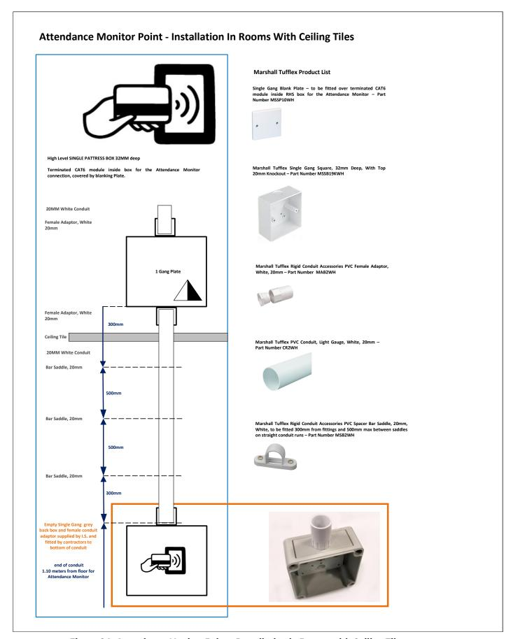
Figure 24: Attendance Monitor Point - Installation in Rooms with Ceiling Tiles
