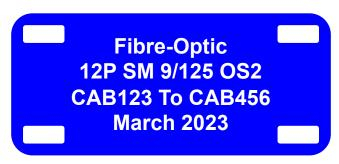
Figure 19: Fibre-Optic Cable Label
