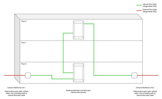
Figure 2: Fibre-Optic Building Feeds and Interconnects
