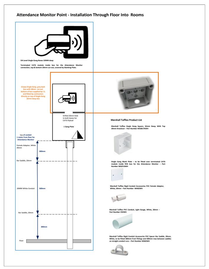
Figure 26: Attendance Monitor Point - Installation Through Floor Into Rooms
