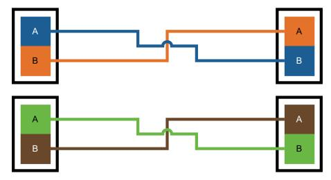
Figure 11: Fibre Core Patch Panel Termination
