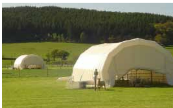
Figure 5. Measuring GHG emissions from sheep grazing different pastures using polytunnels.
