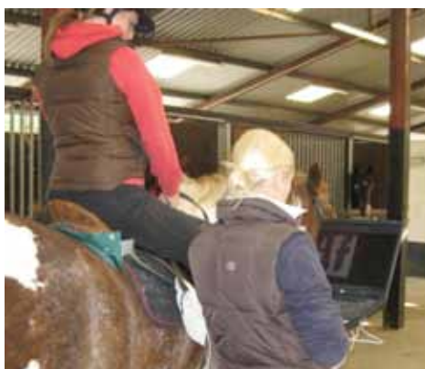
Downloading on to the computer the recording of the relative pressures placed on the horse's back by the rider and saddle, the pressure pad can be seen as the green mat under the back horse's saddle cloth
