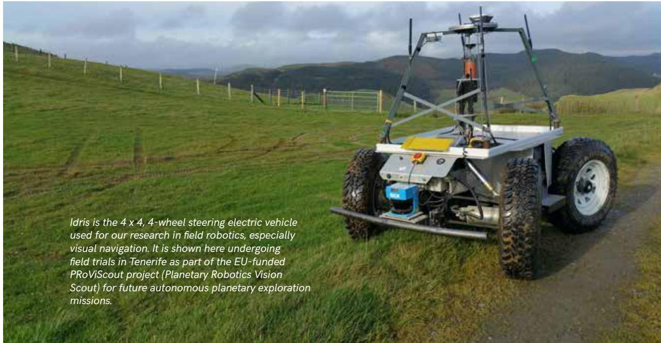
*Idris is the 4 x 4, 4-wheel steering electric vehicle used for our research in field robotics, especially visual navigation. It is shown here undergoing field trials in Tenerife as part of the EU-funded PProViScout project (Planetary Robotics Vision Scout) for future autonomous planetary exploration missions.*
