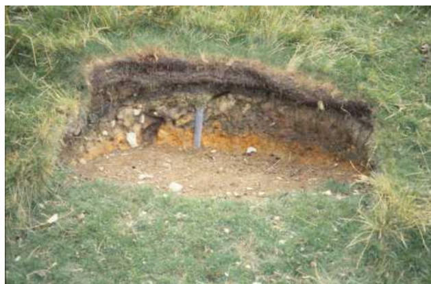
Podzol profile exposed in Sheep nest (ruler 15cm), 1km WSW of Ponterwyd, SN737803, August 1999
