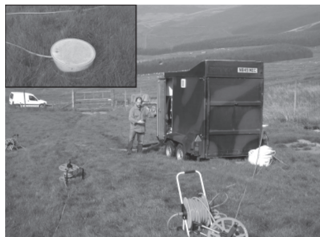
Fig 1 Dr. Nick Ostle of the CEH Lancaster Environment Centre and his ^{13}\text{CO}_2 pulsing system in action at the NERC Soil Biodiversity field site at Sourhope. Inset a close-up view of one of the six pulsing chambers that can be used simultaneously. The cost of ^{13}\text{CO}_2 used for single pulsing experiments can be very high (ca. £30,000).
