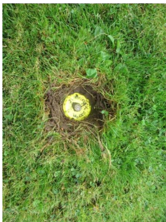
Fig. 1: Yellow plastic disc marker used to mark plot corners. Held in place with a metal nail.
